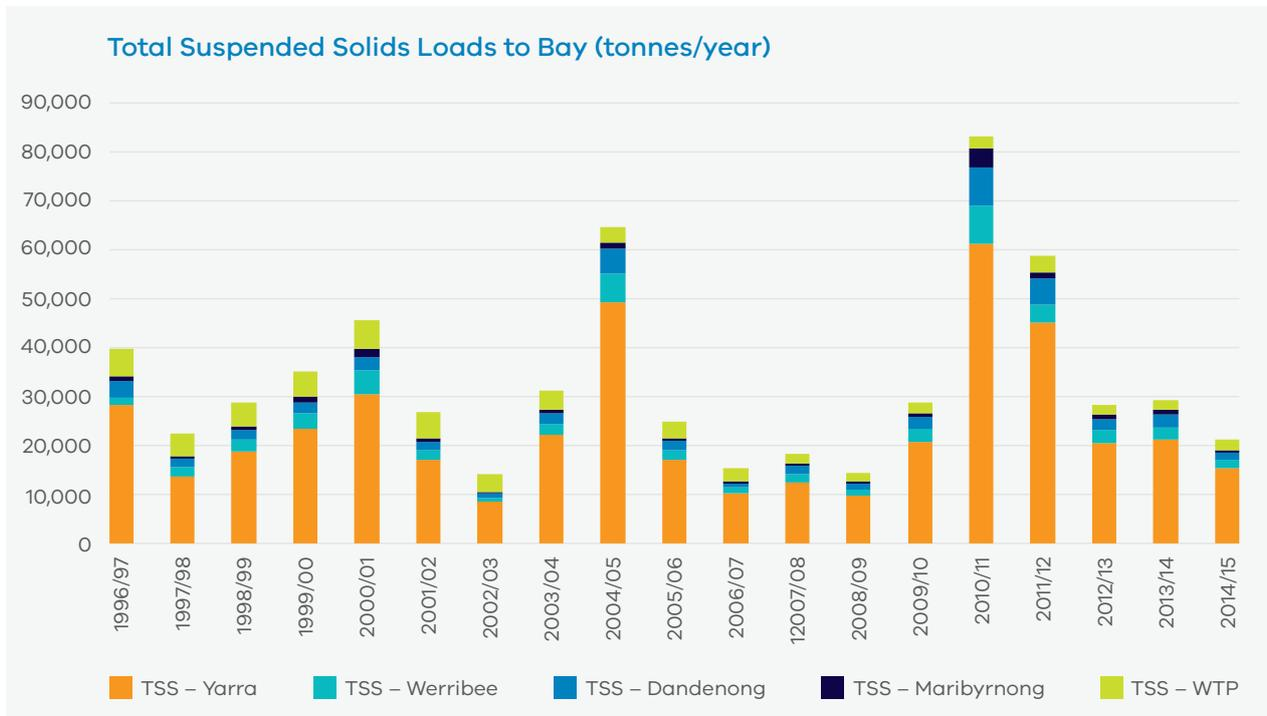
**Figure 9** Estimated annual loads of sediment (total suspended solids, TSS) based on catchment modelling. Loads for Werribee and Dandenong include contributions from smaller rivers and creeks that discharge directly to the Bay in those regions.
