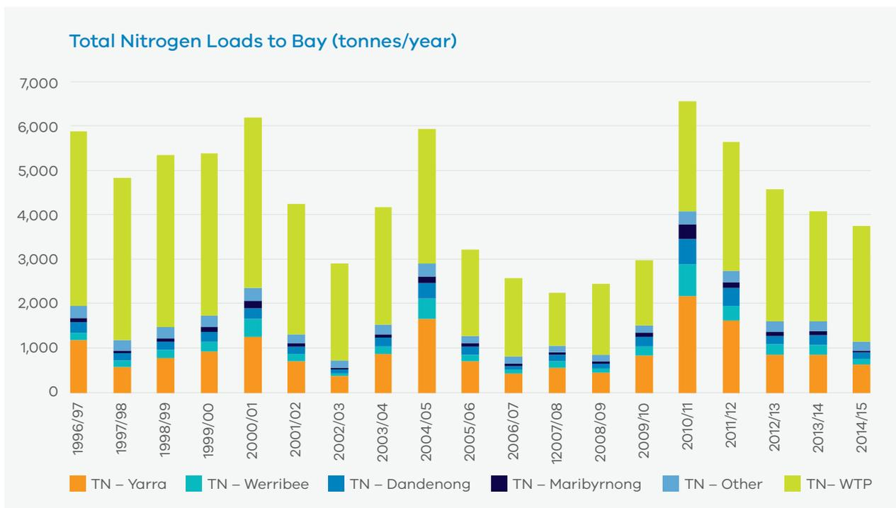
**Figure 7** Estimated annual loads of total nitrogen (TN) based on catchment modelling. Loads for Werribee and Dandenong include contributions from smaller rivers and creeks that discharge directly to the Bay in those regions. 'Other', includes discharges from drains and minor waterways not included in the four major catchments/regions, direct discharge of groundwater and atmospheric deposition to the Bay.
