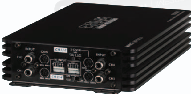
4-CHANNEL MOSFET END PANEL DETAIL
