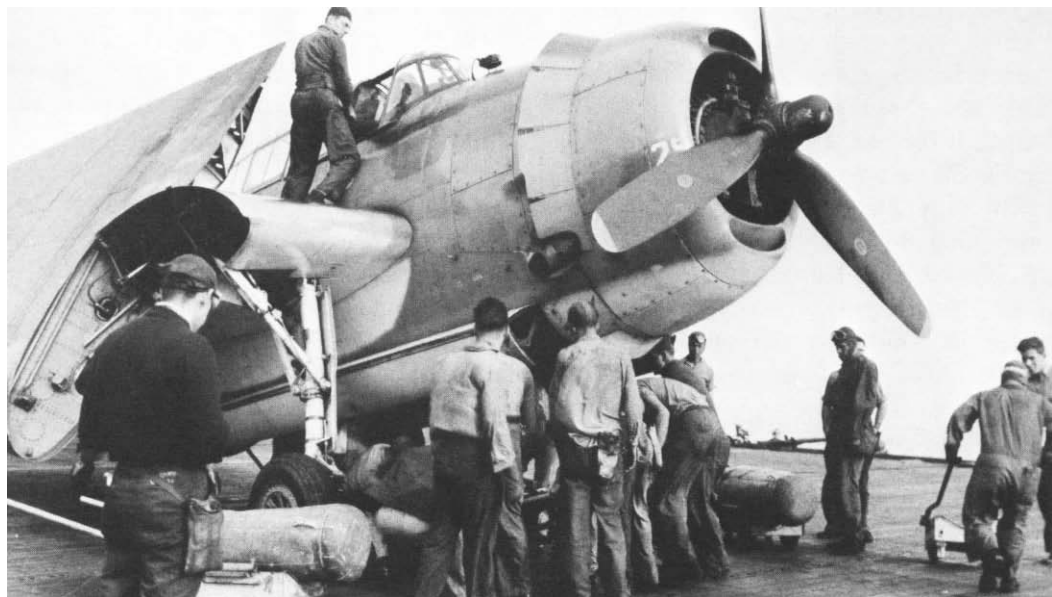
AIR DELIVERY SECTION Marines and ship's crew of USS Sargent Bay load a TBM with supplies to be dropped to Tenth Army troops. (USN 80-G-338840)
