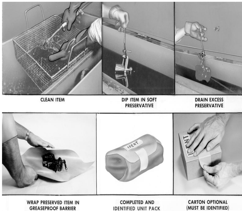
Figure 4-22. Application of Method 20 using a soft film preservative.
