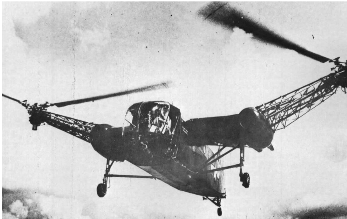
The extended rotor idea of the McDonnell XHJD-1 never proved workable as the aircraft was unstable (National Archives Photo 80-G-395920).
