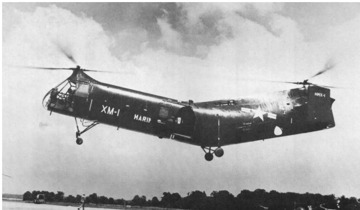
The HRP-2 replaced the HRP-1 and provided greater payload and higher speed (Marine Corps Photo 529983).
