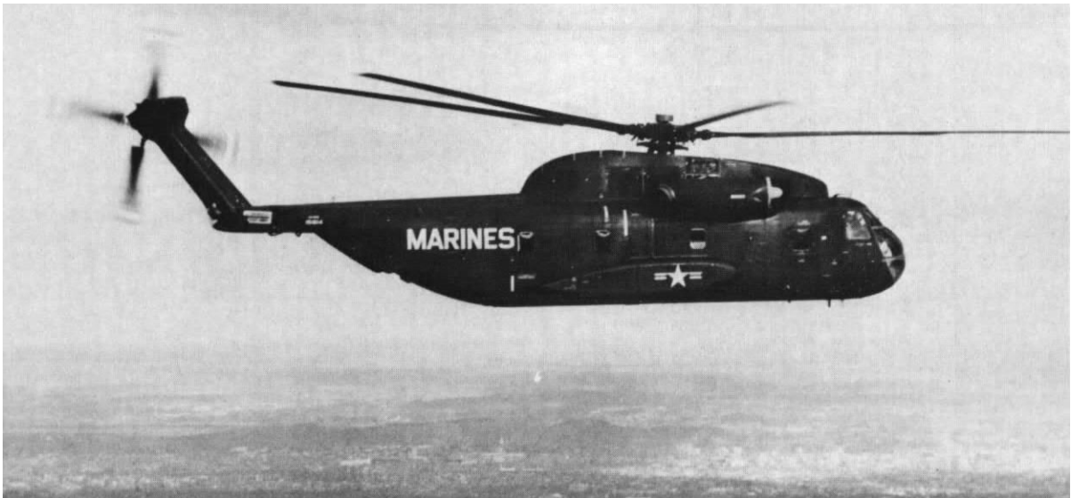
The CH-53A was developed during 1962 and placed in service in 1964. It is a heavy assault transport with a cruising speed of 172 knots and a troop capacity of 38 (Marine Corps Photo A412901).
