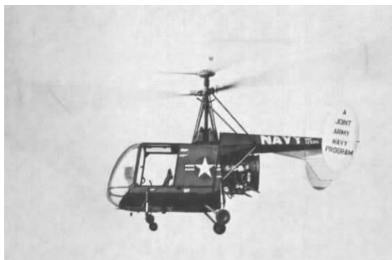
Research in drone helicopters has continued from the days of the autogyro. HTK-1 testing in 1958 led to the conclusion that the major use of drone helicopters would be for cargo transport (Kaman Aircraft Corp. Photo 2570-1).
