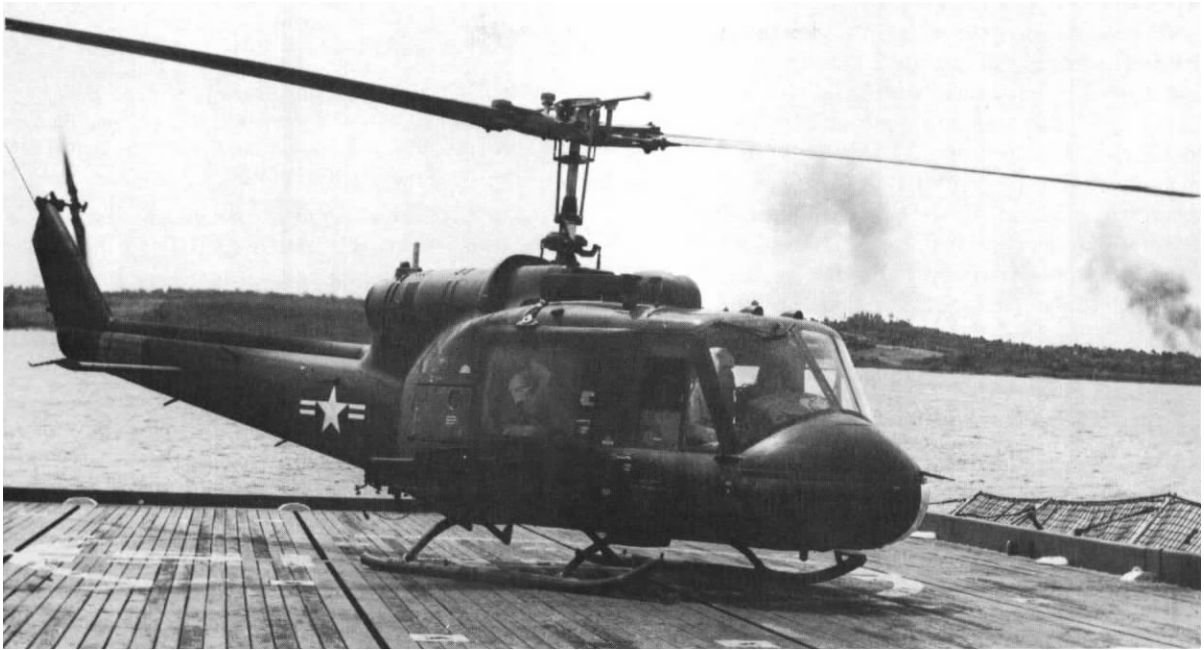
The UH-1E was designed in 1962 and placed into service in 1964. It is the smallest and lightest aircraft in the modern Marine helicopter service.
