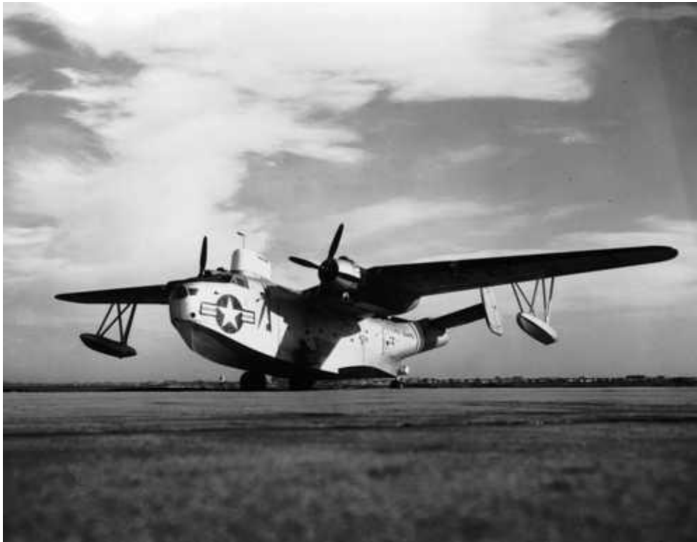
A Coast Guard Martin PBM-5G Mariner. A seaplane such as this crashed while attempting to rescue the crew of a Navy P5M Neptune in 1953 off the coast of China. These large, twin-engine seaplanes were in wide use in the Coast Guard from 1943 through 1956. Note the detachable landing gear.
