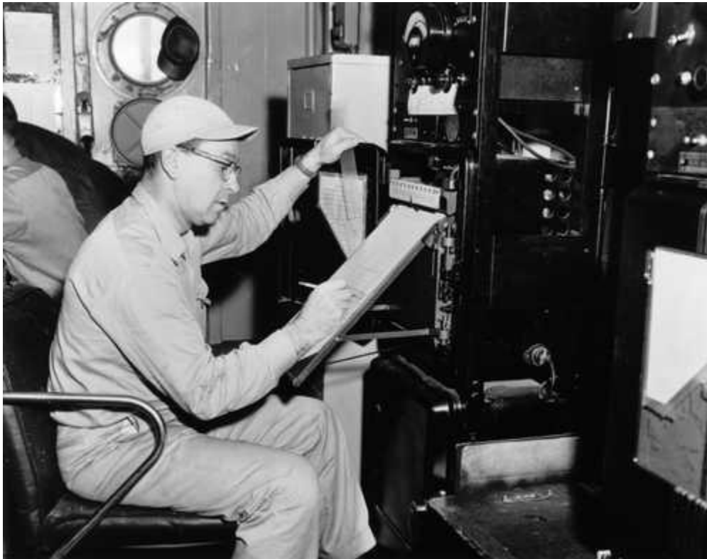
Senior Weather Bureau observer Edward J. Fencil seated at a RADIOSONDE receiver-recorder aboard the cutter Abesecon computes from a continuously moving graphic tape tracings transmitted from a balloon-borne RADIOSONDE transmitter high up in the atmosphere. His computations tell him the pressure, humidity, temperature, and wind velocity at various altitudes the balloon has reached.
