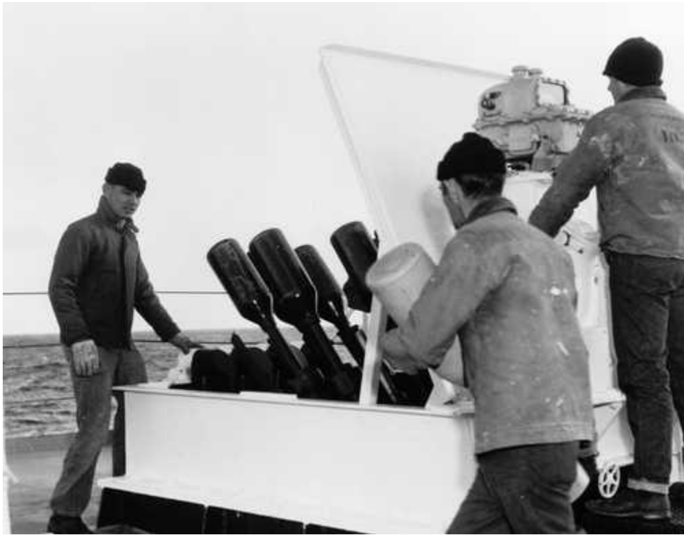
The crew of the Coast Guard cutter Chincoteague rearm the hedgehog anti-submarine mortar. During the Korean conflict every cutter was heavily armed, including anti-aircraft and anti-submarine weapons.
