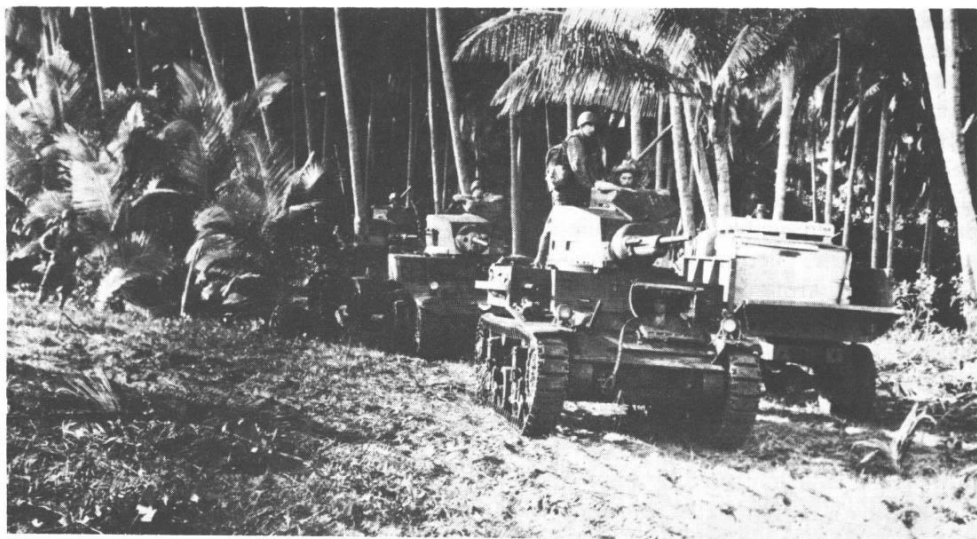
MARINE LIGHT TANKS, mounting machine guns and 37mm cannon, were severely hampered in their operations by the jungle terrain of Guadalcanal. (USN 18525)
