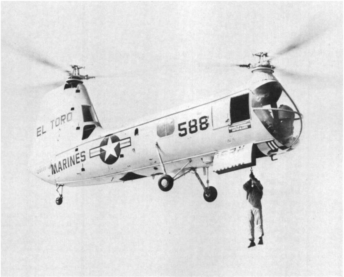
The Piasecki HUP-1, shown practicing a rescue lift, was one of the last helicopters introduced in the 1940s and was the first of the multipurpose helicopters (Marine Corps Photo 529604).
