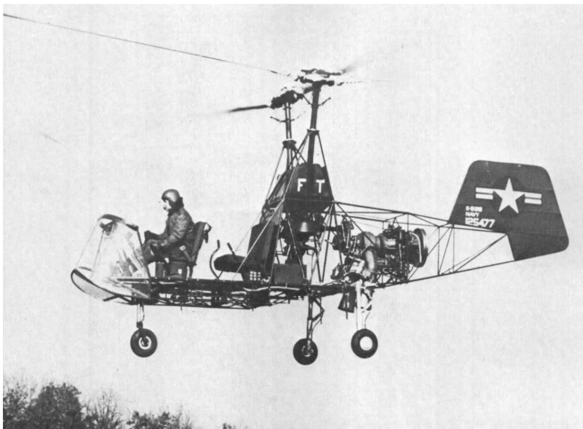
The K-225 was the first turbine-powered helicopter. Built by Kaman, it was powered by a Boeing 502-2 free turbine (Kaman Aerospace Corp. Photo 115-1).
