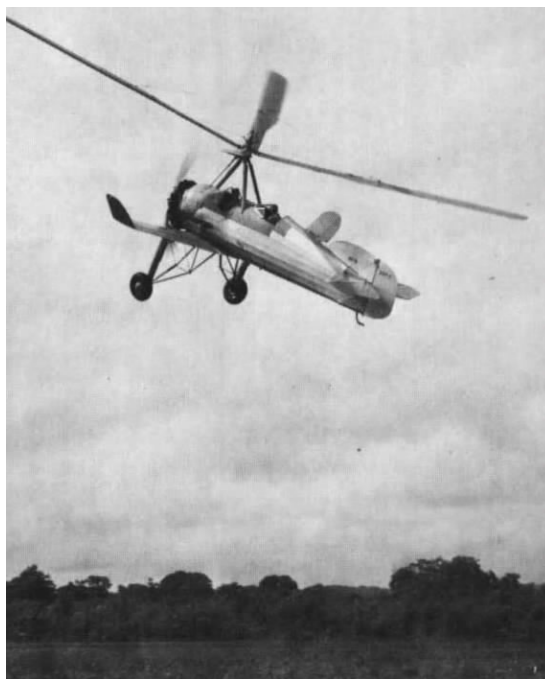
The Pitcairn Autogyro was the first rotary-winged Marine aircraft. Field tested in Nicaragua, it soon disappeared from the active inventory (Marine Corps Photo 515209).
