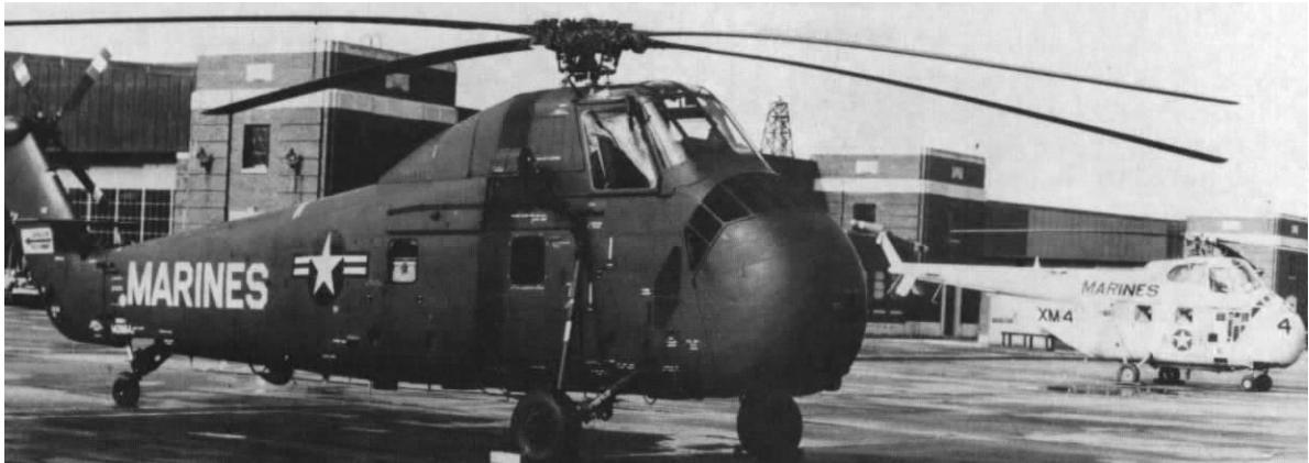
The HUS-1 by Sikorsky was the first major Marine utility helicopter. Its forerunner was the HRS-1 (background) (Marine Corps Photo 529979).
