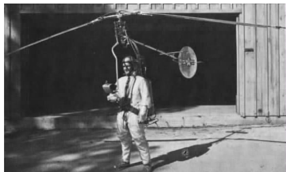
The dream of a one-man, portable, flying machine never materialized. The closest operational device was this Rotorcycle (Navy Photo Np/45/5834).
