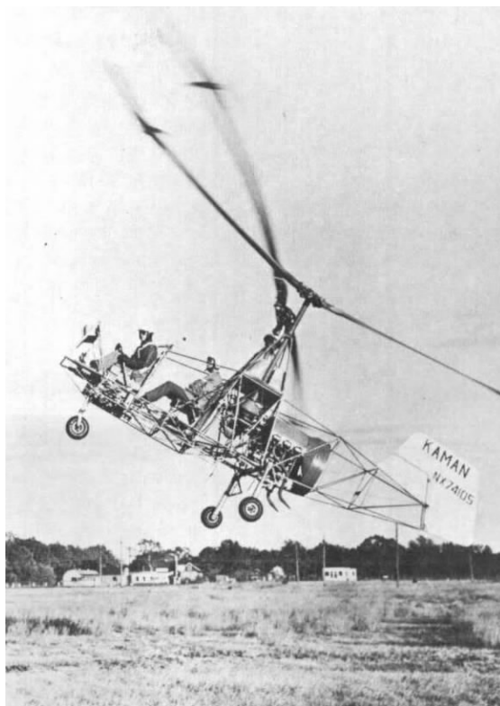
The Kaman K-190 featured twin, intermeshed, two-bladed rotors. Only one model was purchased by the Marine Corps (Kaman Aerospace Corp. photo).
