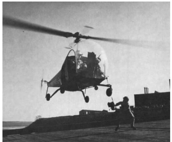
A Bell HTL-5 demonstrates wire laying at Quantico (Marine Corps Photo KV1-4173).
