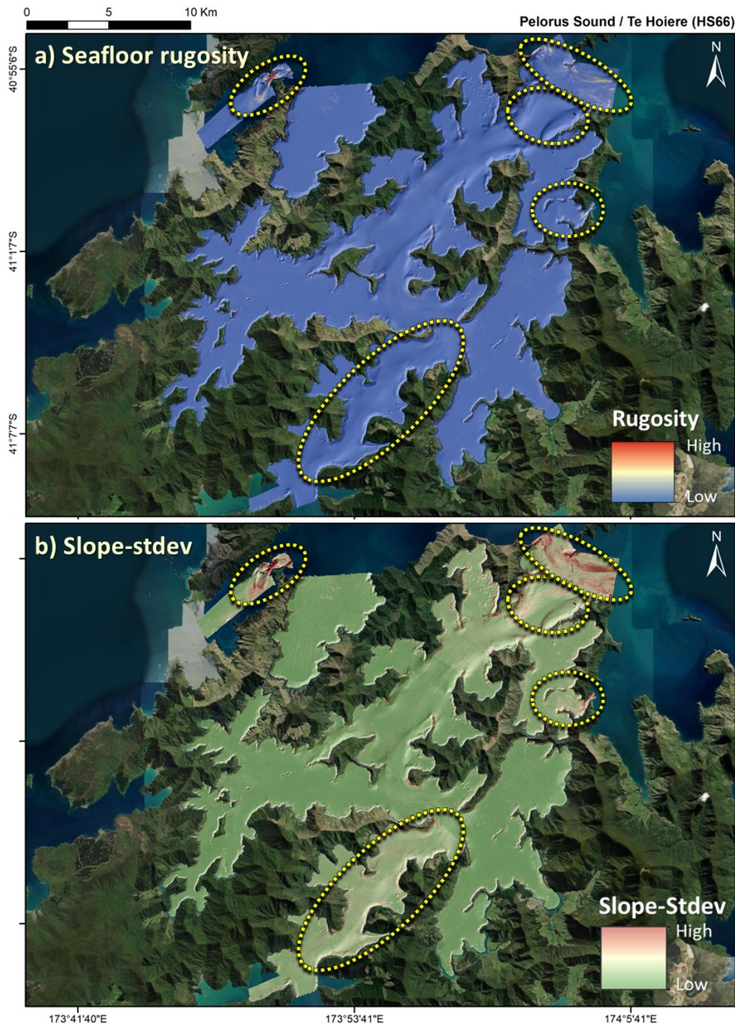
Figure 29. Comparison between seafloor rugosity (a) and the standard deviation of the slope (slope-stdev) (b) across the HS66 survey. Yellow dotted circles highlight areas of comparison, at large spatial scales, where slope-stdev provides significant addition information to the rugosity layer in terms of the roughness of the seafloor. This is very valuable as it can provide considerable insight into the presence of low-relief structure on the seafloor (white-red) such as living and relict biogenic habitats and cobble/rubble.
