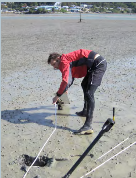
Installing sediment plates at Site B
