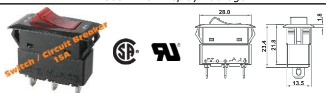
Snap-in mounting circuit breaker/switch (SPST) with neon indicator. 7-16A @ 125/250VAC. Mtg. hole: 30.2 x 14.2mm
