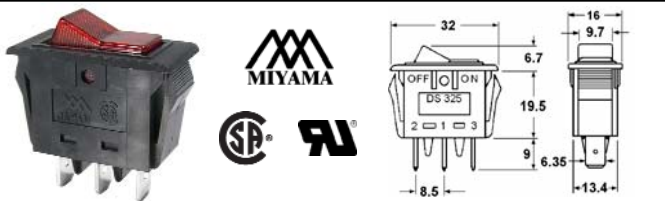
Snap-in mounting with neon indicator. 15A @ 125VAC. Mtg. hole: 30.2 x 14.2mm
