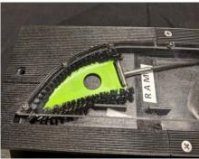
Note: Make sure to push the Dshaped Brush to the end of the channel, moving any debris to the Drain Channel. (*Tile not shown for* clarity)
