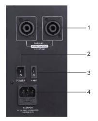
1. Speakon<sup>™</sup> outputs - Parallel outputs for connection to your loudspeakers
