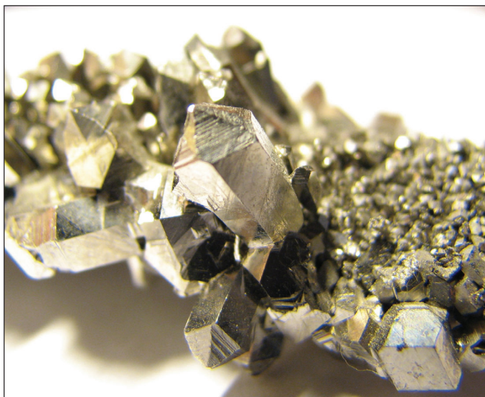
Figure 1. Crystals of refined Nb. Largest crystal in center is 7 mm. Photo by Artem Topchiy (CC-BY-SA-3.0).
