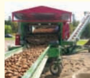
13. A grader removes excessive soil and foreign matter before the potatoes are put into storage.
