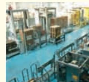
12. Machines pack the bags into cardboard boxes and then onto pallets, which are stored at -23° Celsius until shipped.
