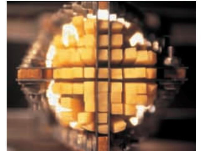
**TOP:** Knives are inserted into the knife box, which is similar to a cannon barrel: potatoes are fired through it.
