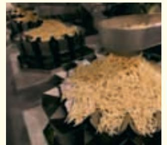
10. The packaging machine weighs out batches of french fries and drops them into plastic bags.
