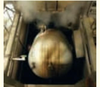
2. After stone removal, high-pressure steam loosens the skins. Automated brush peelers remove remaining skin.
