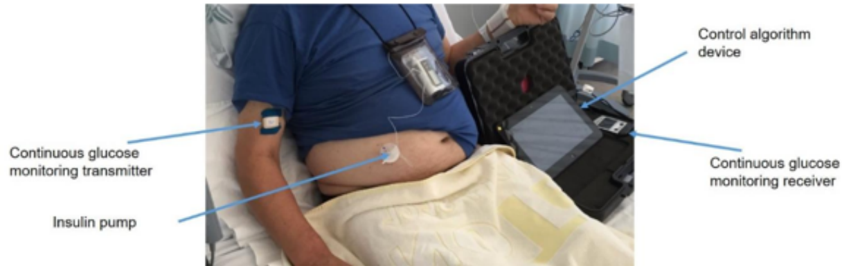
Figure S1. Automated fully closed-loop insulin delivery prototype (FlorenceD2W-T2) used in the study (photo obtained with consent).
