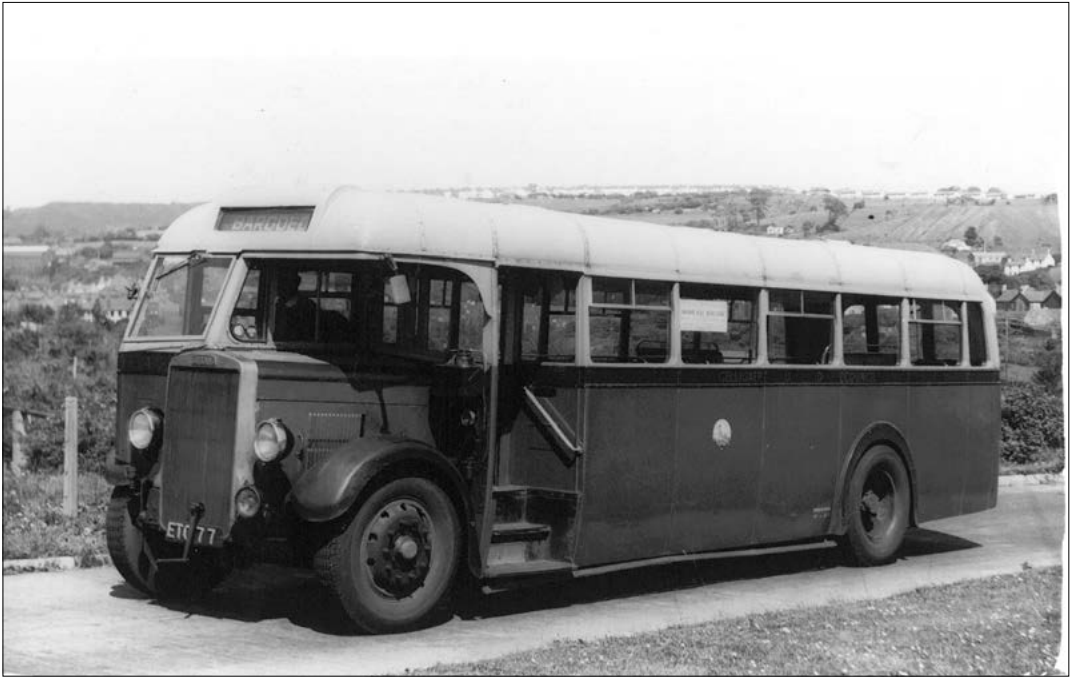
Strachan-bodied Leyland TS8 of 1939 No.4 was rebuilt by Bruce Coachworks in 1950 with a B34F body and is seen here at the Tiryberth garage in reconstructed condition.
