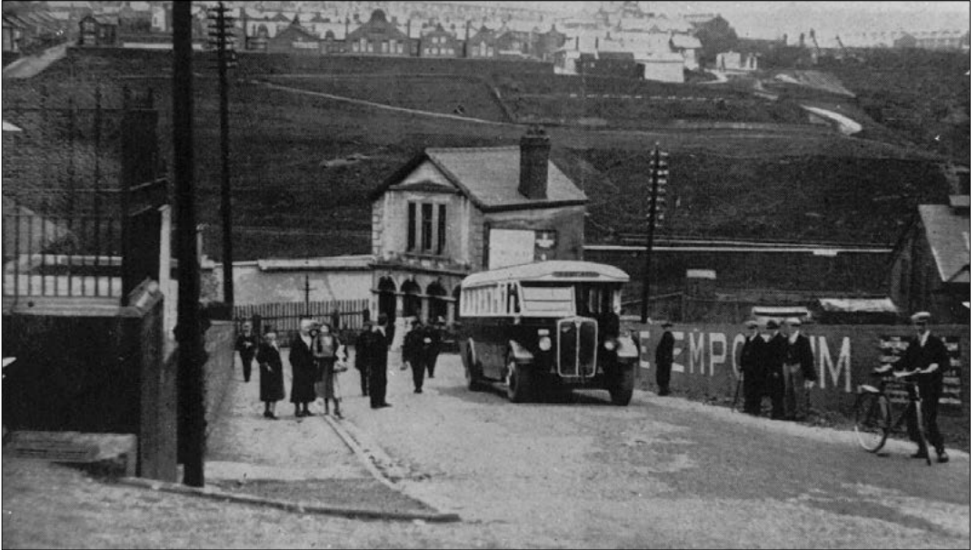
Metcalfe-bodied AEC Regal No.8 (TG 1154), delivered in 1931, is seen on trials at Bargoed.
