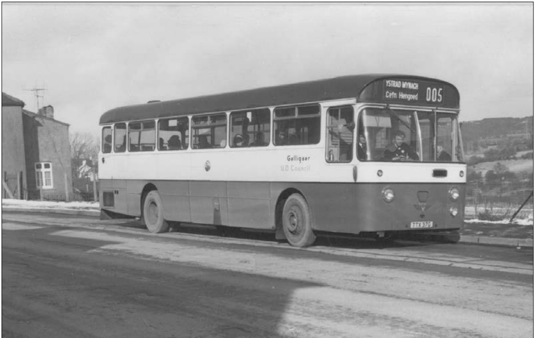
Dual-entrance Willowbrook-bodied AEC Swift, No.37 (TTX 37G) is seen here at Pengam in 1969 en route for Ystrad Mynach.
