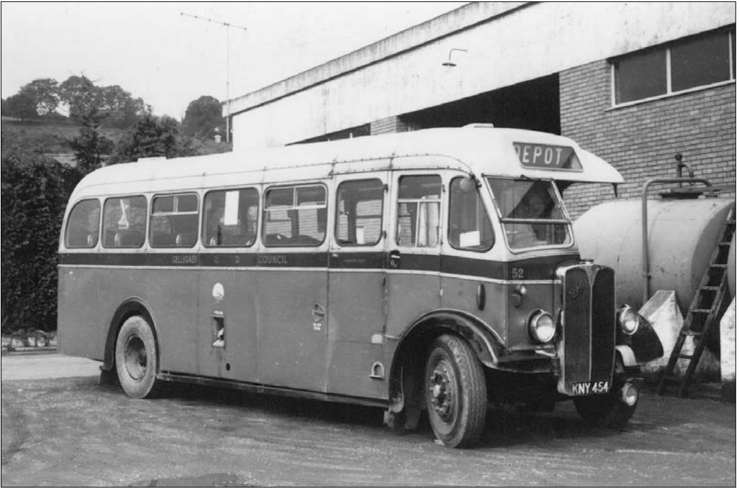
One of the AEC Regal/Duples, No.17, later 2 and here temporarily 52, is seen as late as 1967, shortly before withdrawal, at Tiryberth: the body was rebuilt by Longwell Green in 1958-9 and the outswEEP of the skirt removed.
