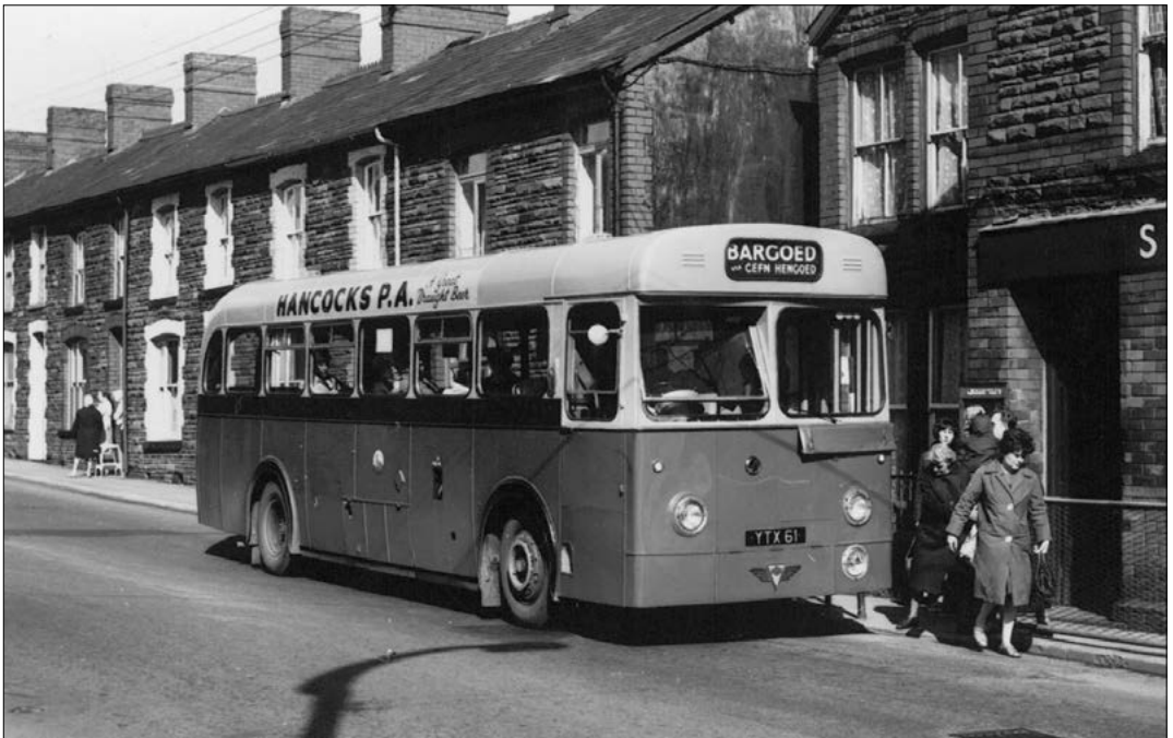
By 1967, when Longwell Green-bodied Reliance No.4 was seen at Gilfach on the Cefn Hengoed service, the AEC badge had been moved to the bottom of the front panel.
