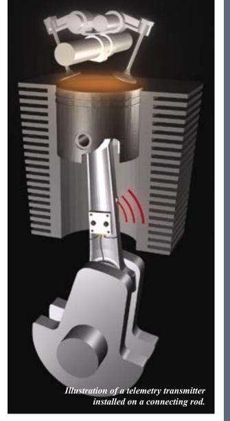
of wireless telemetry to record data within the engine in Miers' laboratory.
