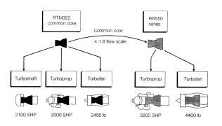
Figure 1-3. Rolls Royce's aircraft engine family; adapted from (Rothwell & Gardiner, 1990).
