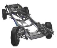
Figure 1-2. Rolling chassis automotive module; adapted from (Kimberly, 1999).
