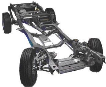
Figure 1-2. Rolling chassis automotive module; adapted from (Kimberly, 1999).
