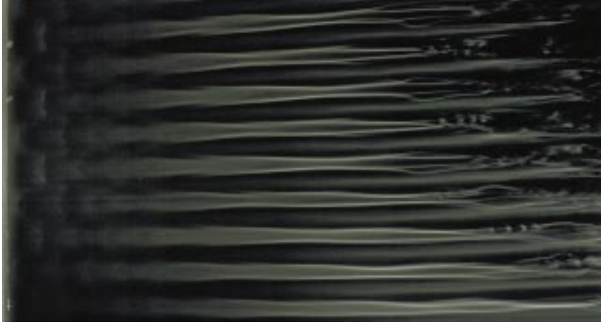
Figure 2: A flow visualization photograph showing oblique transition in a flat plate boundary layer flow. The free stream velocity is 8.4 m/s and the flow is from left to right. The picture is approximately 220 mm wide and 420 mm long. The left hand side is 240 mm from the plate leading edge (flow visualization by Elofsson).
