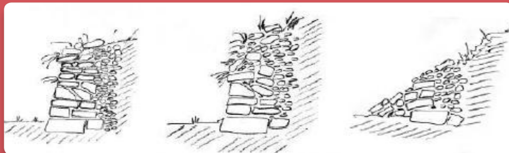
Localized degradation of wall top
