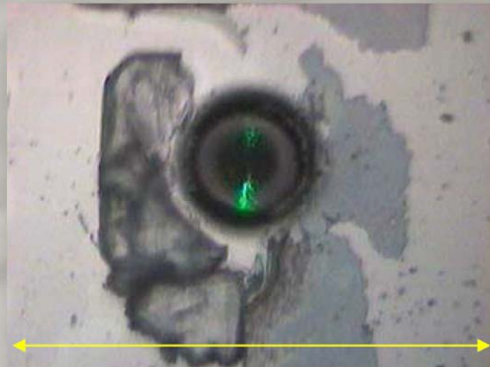
Figure 1 Microscope view of the inkjet hole using a 20X lens. Scale (yellow) is 250um. The green spot is the laser focus.
