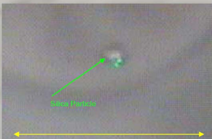
Figure 3 20M microscope image of a silica particle found in the opening. Scale (yellow) is 50um.
