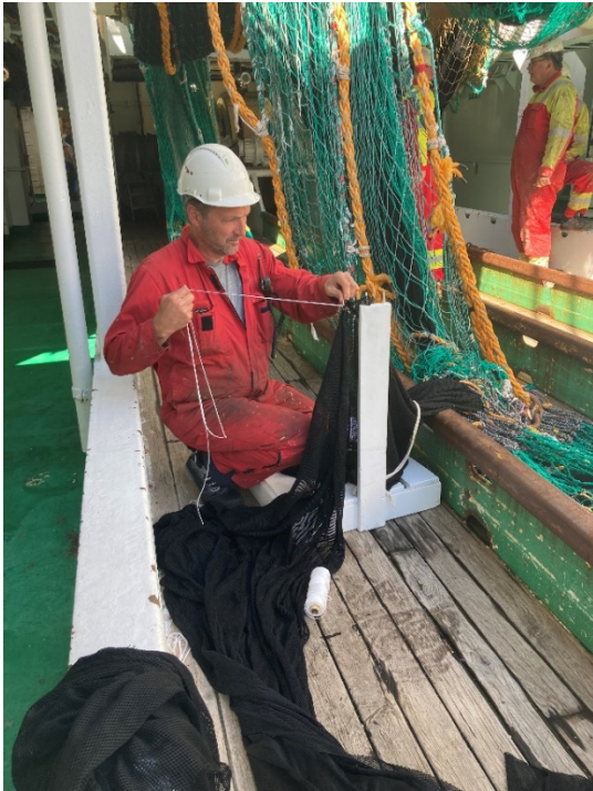
The fishing master repairing the fine meshed trawl. Photo: Webjørn Melle.
