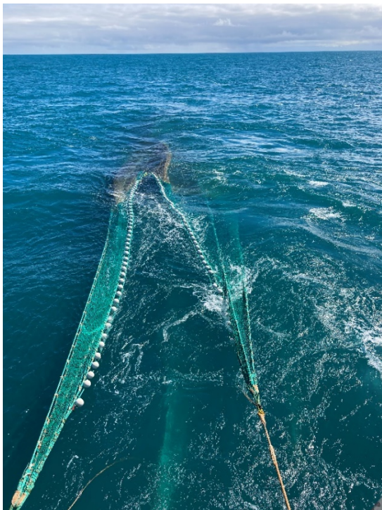
Shooting the 280 Egersund Micronekton trawl. Opening area about 345 m 2 , 16-mm stretched mesh size (7x7 mm mesh opening). Photo: Webjørn Melle.
