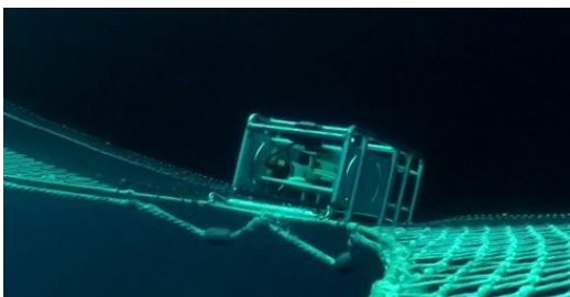
The ADCP attached to the trawl during a haul. Photo: Mel Underwood.
