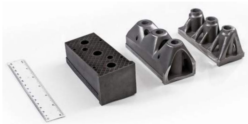
Fig. 4 A punch in an industrial production tool for the stamping of 1 mm thick hot-dip galvanised DP600 sheet. From left to right: the conventional design with a honeycomb inner structure, topology optimised with LS-TaSC, and topology optimised using Siemens NX12. All three punches are additively manufactured in maraging steel 1.2709 (Courtesy Nader Asnafi)
