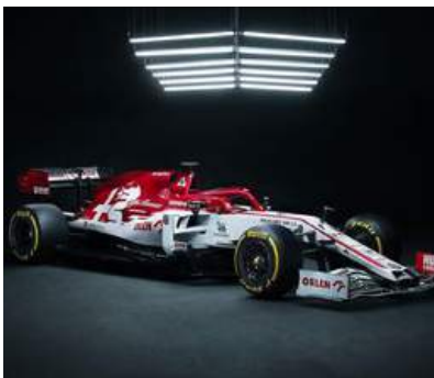
The C39 F1 race car features 143 additively manufactured parts, saving 2% of the car's weight (Courtesy Alfa Romeo Racing Orlen)
