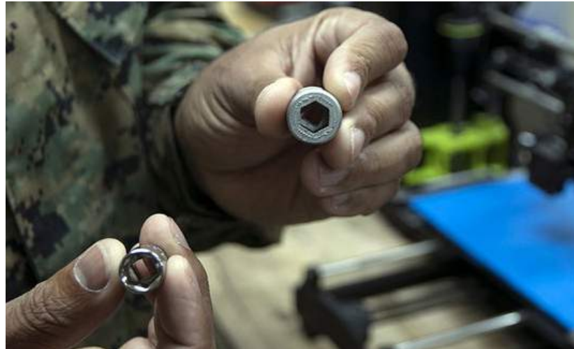
The socket on the right was made with the unit's new Markforged Metal X (Courtesy M M Burke/Stars and Stripes)
