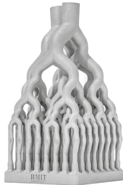
Additively manufactured Ti-6Al-4V dual fluid flow distributor and mixer comprising of 64 mixed outlets (Courtesy RMIT University)
