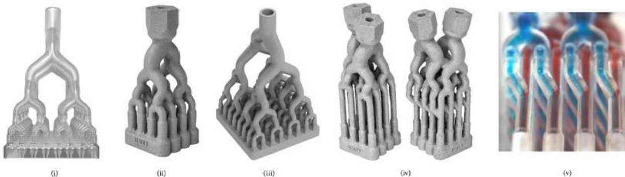
Flow distributor and mixer devices (i) Six-stage polymer flow distributor (64 outlets) (ii) Four-stage Inconel 625 flow distributor (16 outlets) (iii) Six-stage Inconel 625 flow distributor (64 outlets) (iv) Four-stage Inconel 625 dual fluid flow distributor and mixer (16 outlets) and (v) Four-stage dual fluid flow distributor and mixer in operation (Courtesy RMIT)
