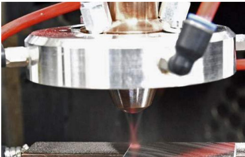
Fig. 6 Three jet nozzles for Directed Energy Deposition with additional shielding gas shroud
