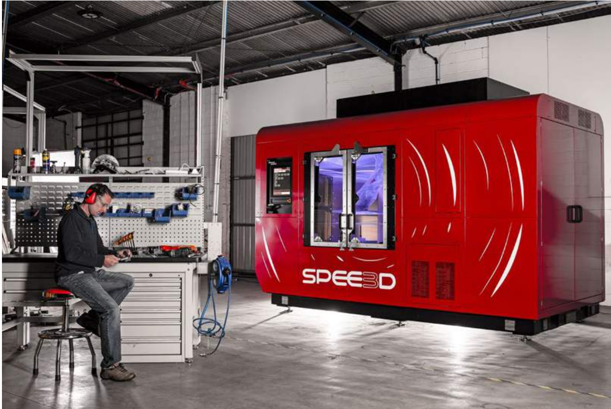
Fig. 5 The WarpSPEE3D system, released in 2019, has a build volume of 1 m diameter by 0.7 m and was designed with robustness on a manufacturing floor in mind
