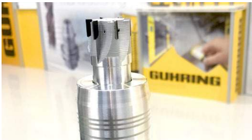
The additively manufactured H13 tool steel milling cutter was produced using a Markforged Metal X system (Courtesy Markforged)
