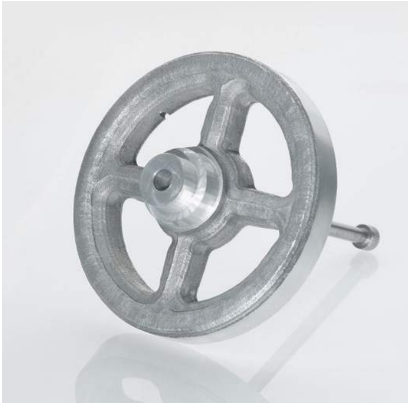
Fig. 7 This aluminium part is a replacement drive wheel for an air compressor. This was an early demonstration of SPEE3D's capability to produce critical replacement components on-demand. It weighs 200 g and took less than eight minutes to produce
