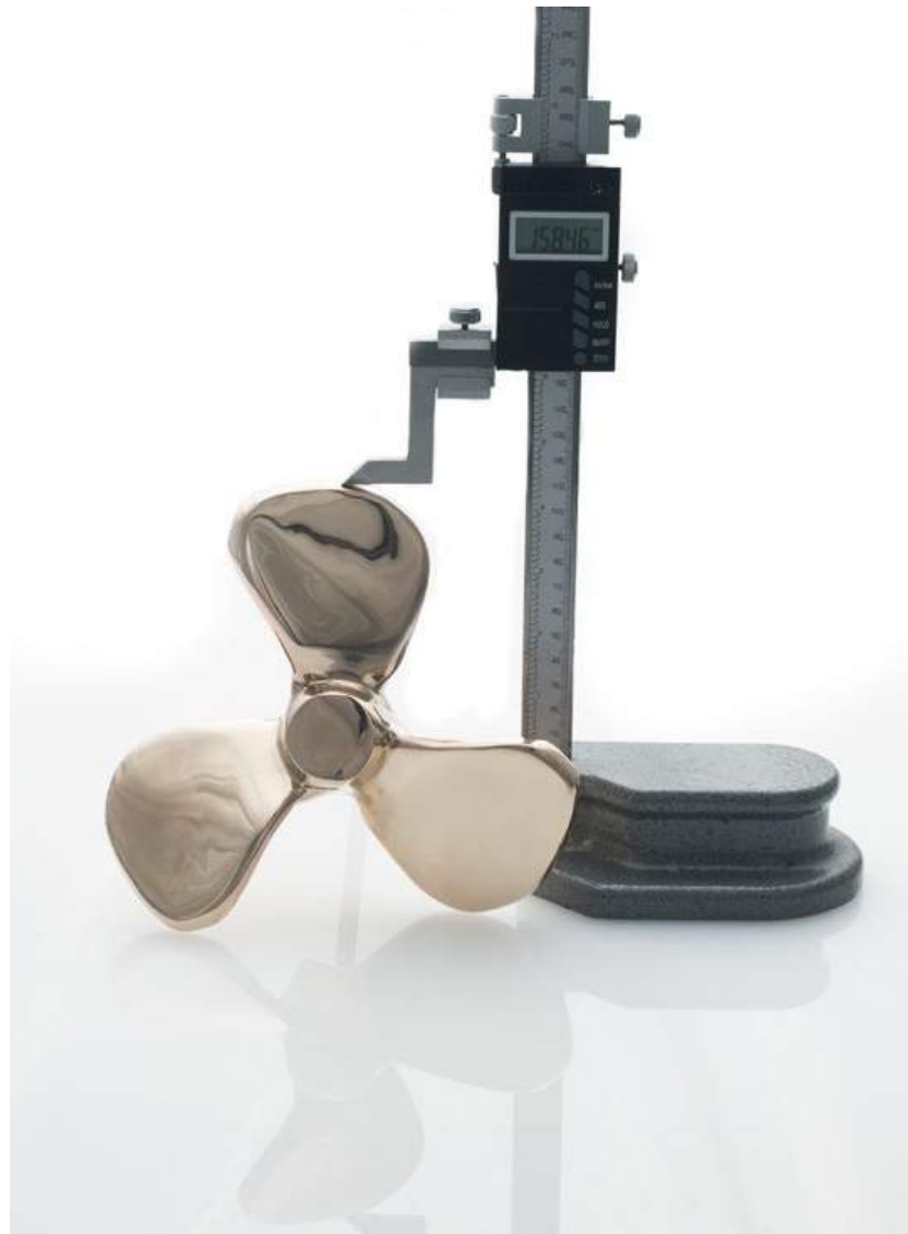
Fig. 6 Rather than focus on exotic materials, SPEE3D's focus has been on the larger markets such as aluminium and copper. This aluminium bronze propeller is corrosion resistant in sea water and naturally anti-fouling, making it ideal for marine applications. The part weighs 1.4 kg and took sixteen minutes to build
