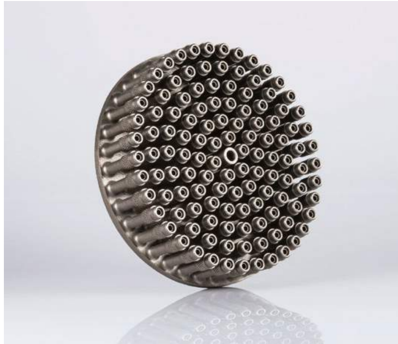
Fig. 3 An Ariane 6 Vinci Engine injector printed as one single piece, including 8000 holes, using Laser Powder Bed Fusion (Courtesy EOS)
