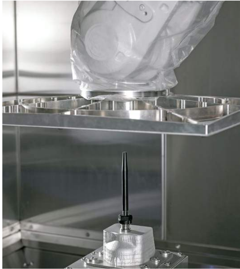
Fig. 4 To most Cold Spray users, the SPEE3D machine design appears counter-intuitive. The nozzle is fixed at the base of the machine and a six-axis robot controls, rotates and orientates the build platform
