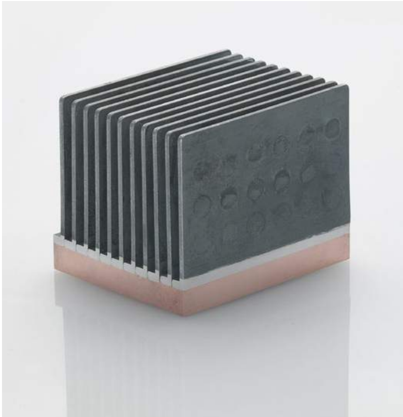
Fig. 12 A multi-material heat sink created by depositing copper powder onto aluminium fins to create a heat sink that is high performance, low weight and inexpensive to produce. This 200 g part weight took two minutes to produce
