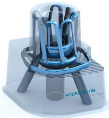
Fig. 5. Core for the injection moulding of a medical container: Cooling performance was improved by 15% and cycle time was reduced by 8%. After optimisation, the core was additively manufactured in a voestalpine material [Courtesy Anton Alveflo]
