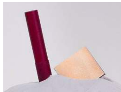
The two AM test parts anodised in red and gold (Courtesy Fehrmann Alloys)
