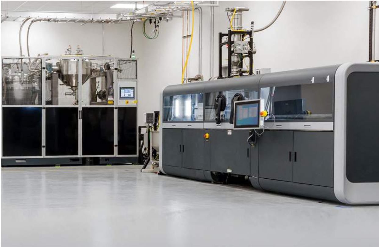
Fig. 5 Binder Jetting processes are viewed as having significant potential in moving metal AM towards industrial production, as can be seen at Indo-MIM's metal Binder Jetting operation in San Antonio, Texas [Courtesy Indo-MIM Inc]
