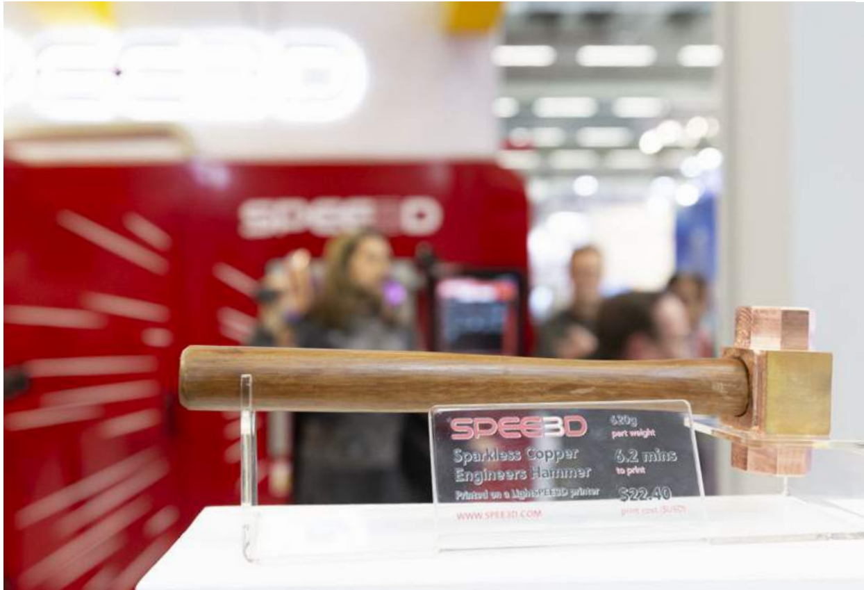
Fig. 11 At Formnext 2019 the SPEE3D team additively manufactured sparkless copper hammer heads in six minutes apiece, to showcase the scalable capabilities of the SPEE3DCell
