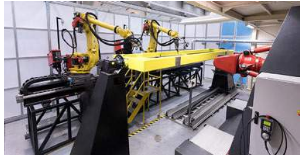
The LASIMM project has developed a fully functional prototype of a multi-robot additive and subtractive manufacturing machine (Courtesy LASIMM Project)
