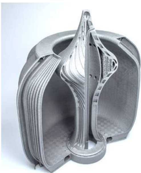
This prototype of the aerospike engine has already been tested by project researchers on the test stand of the Institute of Aerospace Engineering at TU Dresden (Courtesy Fraunhofer IWS)
