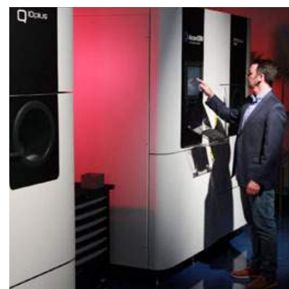
Amplify Additive manufactures titanium orthopaedic implants using three Arcam EBM Q10plus machines (Courtesy Amplify Additive)
