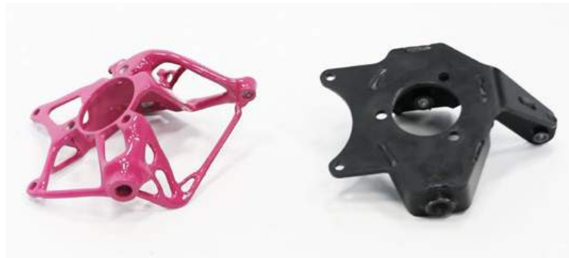
The metal additively manufactured steering knuckle (left) weighed 36% less than the conventionally produced part (right) (Courtesy XponentialWorks)
