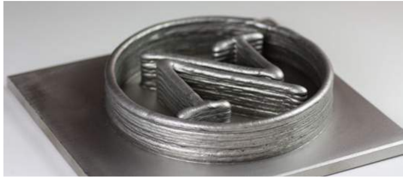
Nordmetall logo additively manufactured on the Gefertec arc 403 system. (Courtesy Gefertec GmbH/Nordmetall GmbH)
