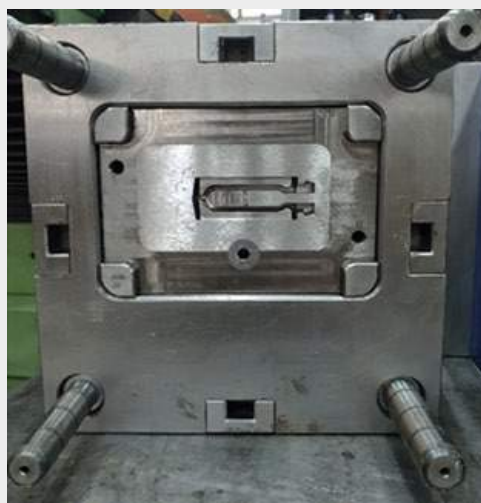
Fig. 11 The improvements achieved with the cooling and topology optimised inserts additively manufactured from AM Corrax (Courtesy Anton Alveflo)
