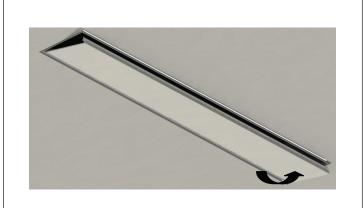
**STEP 8.** Re-attach lens. Start with one side first and close the other side starting from the corner.
