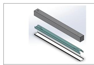
**STEP 3.** Remove reflector mounting screws and reflector. Note fixtures with optional emergency pack have a test switch and indicator light mounted on the reflector.
