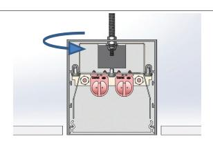
**STEP 5.** Once fixture is parallel with drywall insert second nut (supplied by other) through the fixture and fasten to fix fixture in place. Repeat steps 4 & 5 with remaining mounting locations until fixture is parallel along entire length.
