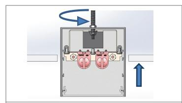
**STEP 4.** Bring electrical supply to the fixture as needed. Make sure to feed ready rod (by others) through mounting locations and adjust nut to ensure fixture is parallel with drywall, insert fixture all the way through the opening in the ceiling.
