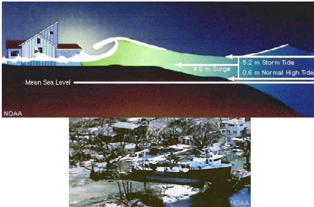
Fig. 10.83. Conceptual model of storm surge and photograph of boat carried inland by storm surge.
