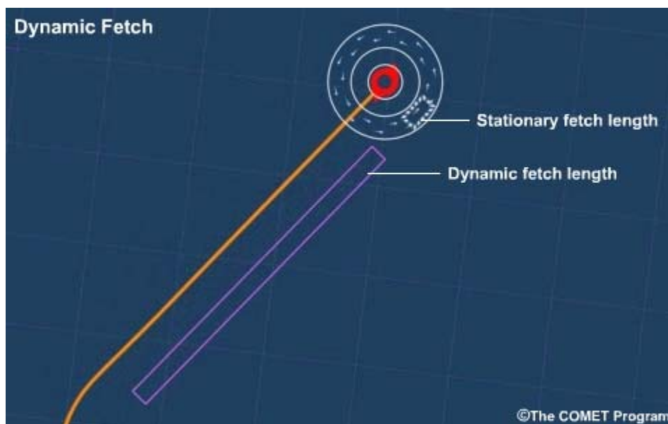
Fig. 10.88. Conceptual model of a tropical cyclone with a straight storm path and a fetch in the right of track (outlined with a dotted white line). Waves within the dotted line experience a longer period of wind forcing; the distance over which they grow is called the effective or dynamic fetch (purple outline).
