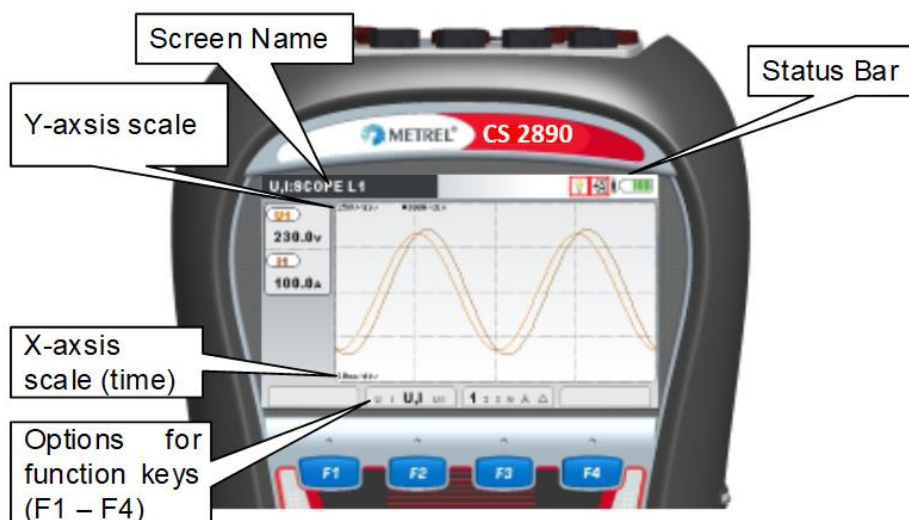
Figure 24: Common display symbols and labels on SCOPE screen
