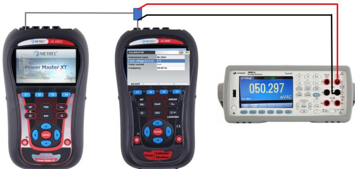
Figure 17: Connection diagram for current adjustment procedure using substandard Volt-meter
