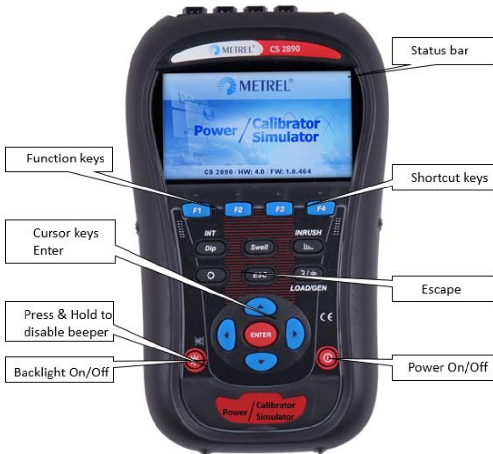
Figure 23: Power Simulator Display symbols and keys description
