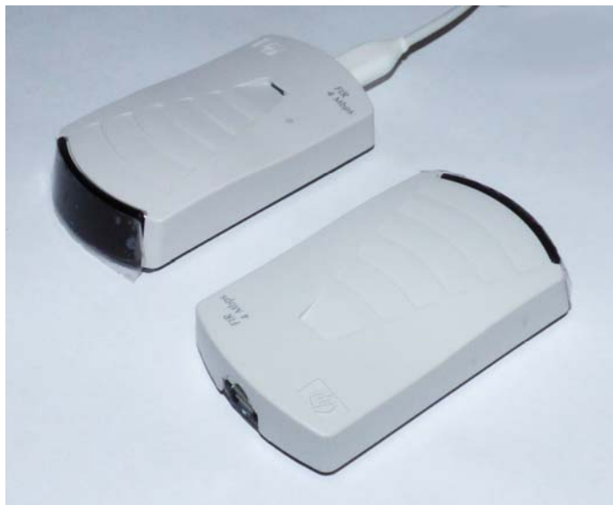
Figure 16: Finished: two variants with the integrated USB-TTL converter board. The rear case has a small hole to reach the reset pin of the Arduino for reprogramming. This is only needed if you want to modify the firmware later without opening the case.
