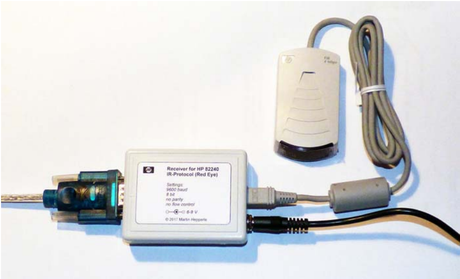
Figure 20: This “RedEye” receiver has a serial interface and connects to the infra-red receiver. An external 6 V power supply is connected to the Arduino’s RAW input.
