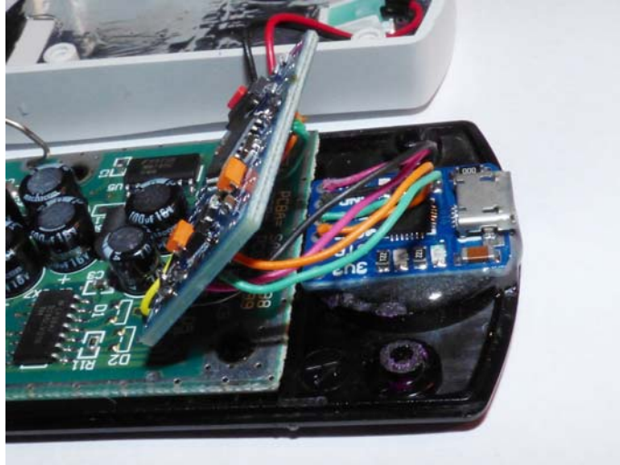
Figure 15: Phew, almost finished: USB-TTL converter board and Arduino Pro Mini connected. The Arduino can be held in place by double sided self adhesive foam tape or glue. The USB-TTL converter PCB has been glued onto the roughened base plate with 5-Minute Epoxy. Make sure that there is sufficient insulation between the PCBs.
