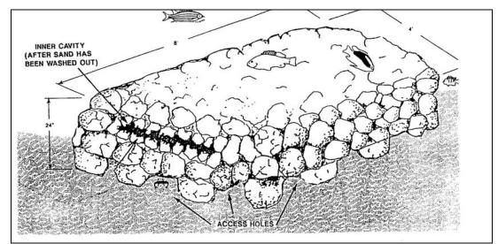
**Figure 4:** Reef Replacement Module (R) diagram(Selby and Associates, Sunny Isles Artificial Reef Monitoring Program: 8<sup>th</sup> Quarterly Report, 1994).
