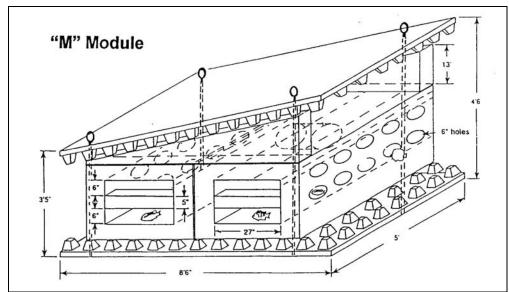
**Figure 3**. Module Design (M) diagram (Selby and Associates, Sunny Isles Artificial Reef Monitoring Program: 8<sup>th</sup> Quarterly Report, 1994).
