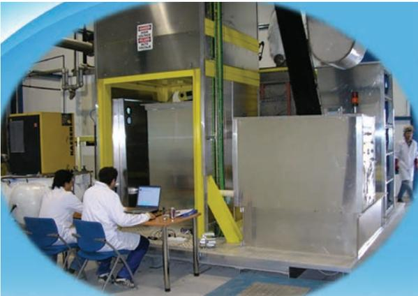
Miami-Dade County's Water and Sewer Department implemented a Plasma Energy Arc Process (PEAP) pilot that uses a new technology to reduce the volume of solid waste 95% while creating syngas (a mix of hydrogen, methane, and carbon monoxide) that can be burned for energy and steam used to process wastewater. The pilot has identified a substantially cheaper way to process biosolids that cuts disposal costs and emissions.
