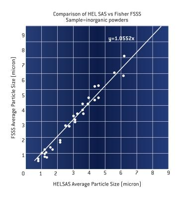
Comparison trials between the HEL SAS and Fisher FSSS have been carried out using a variety of samples. The graphs above compare the mean particle size data from the two instruments on powders of different sizes. One plot is based on results for inorganic (mainly
