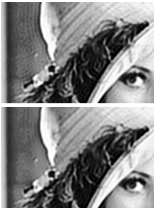
Fig. 4. Deringing via the proposed method. Distorted ( top ) and restored ( bottom ) image. The regularization parameter was set to the minimal value that visually suppresses the artifact. Distorted image: PSNR=30.78, SSIM=0.763. Restored image: PSNR=30.87, SSIM=0.781.
