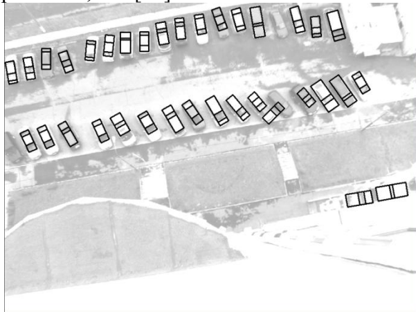
Fig. 1. Detection of passenger vehicles on digital images of optical remote sensing of the Earth.
