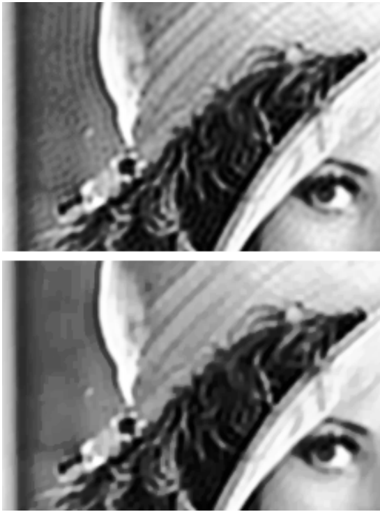
Fig. 2. Deringing via TV minimization. Distorted ( top ) and restored ( bottom ) image. The regularization parameter was set to the minimal value that visually suppresses the artifact. Distorted image: PSNR=30.78dB, SSIM=0.763. Restored image: PSNR=30.82dB, SSIM=0.778.
