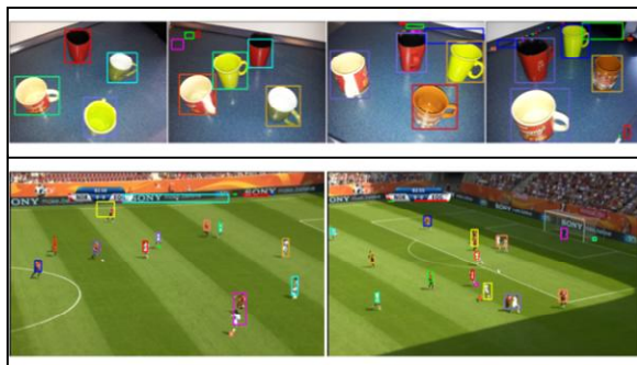
Fig. 3: Results of the programs with the highest fitness for cup (top) and player detection (bottom).
