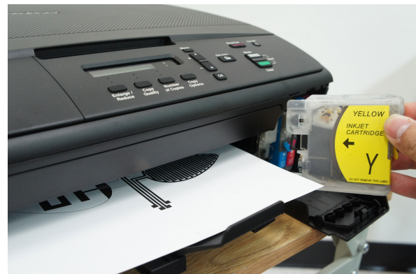
Figure 1. Silver nanoparticle ink is injected into an empty cartridge and used in conjunction with an off-the-shelf inkjet printer to enable ‘instant inkjet circuit’ prototyping.
