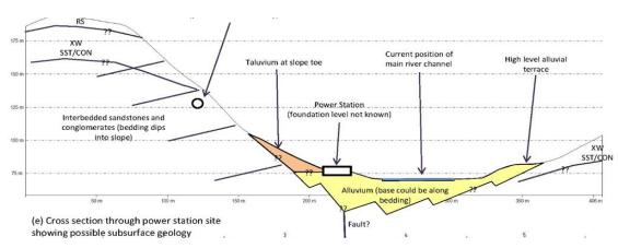
Figure 2-17 Geology at the Powerhouse site
