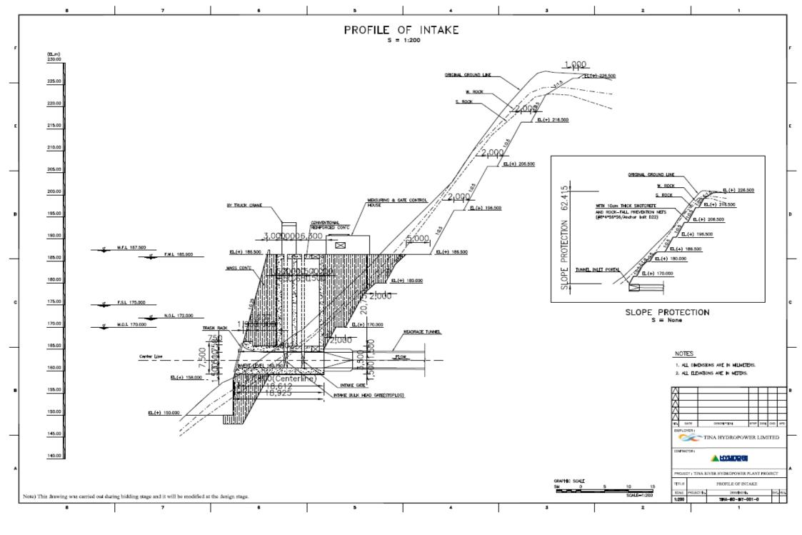
Figure 2-15 Profile of intak
