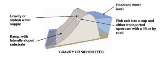
Figure 11-5 An example of Trap and Haul system
