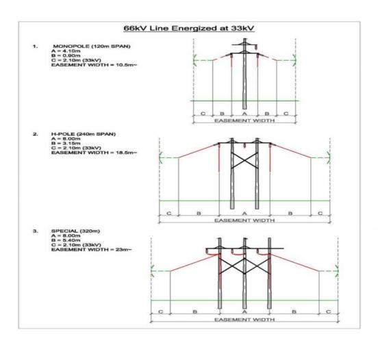
Figure 2-20 Examples of transmission line pylons
