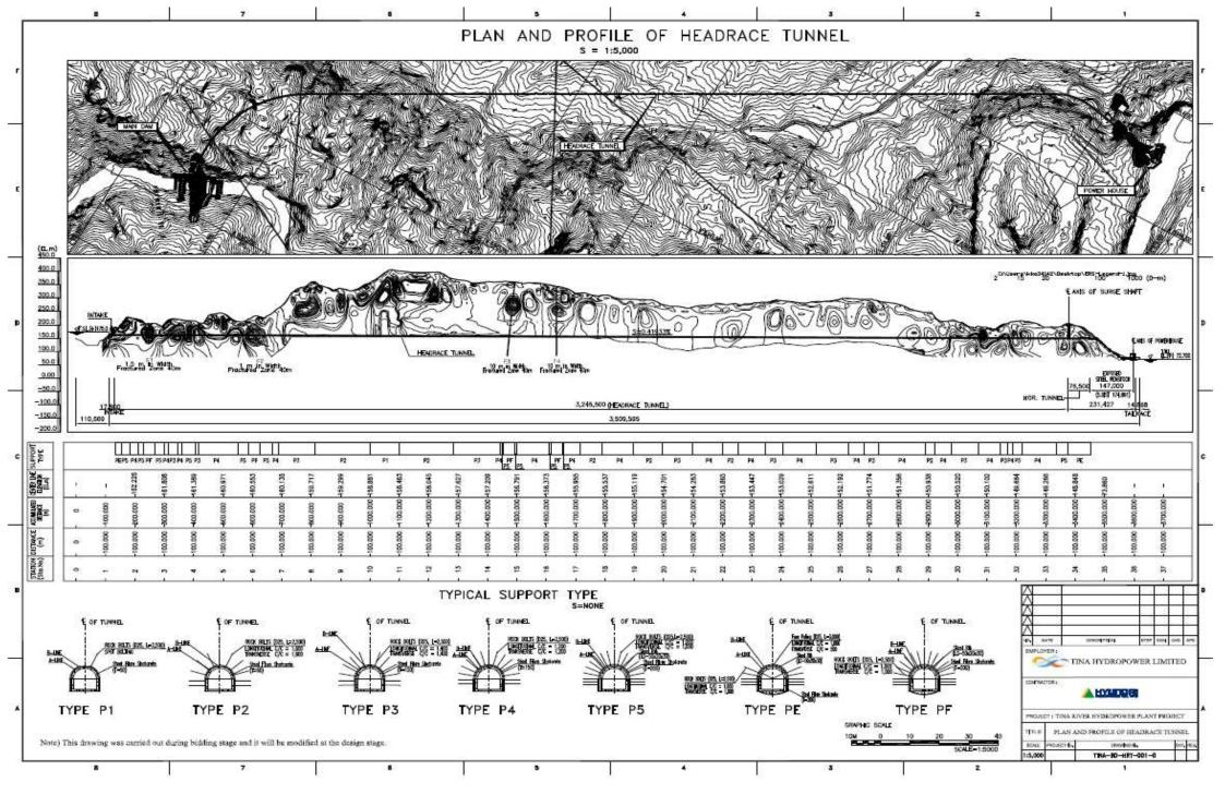
Figure 2-16 Plan and Profile of headrace tunnel
