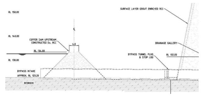
Figure 2-12 Diversion by-pass intake and by-pass plug
