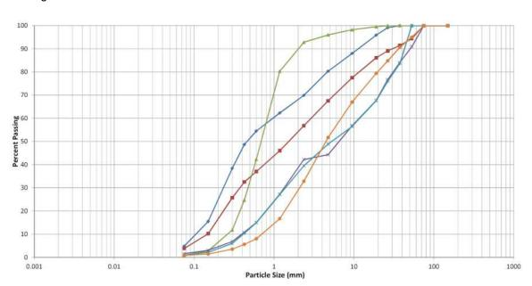
Figure 5-12 Particle size distribution of bed load sediment and alluvial bars in the Tina River
