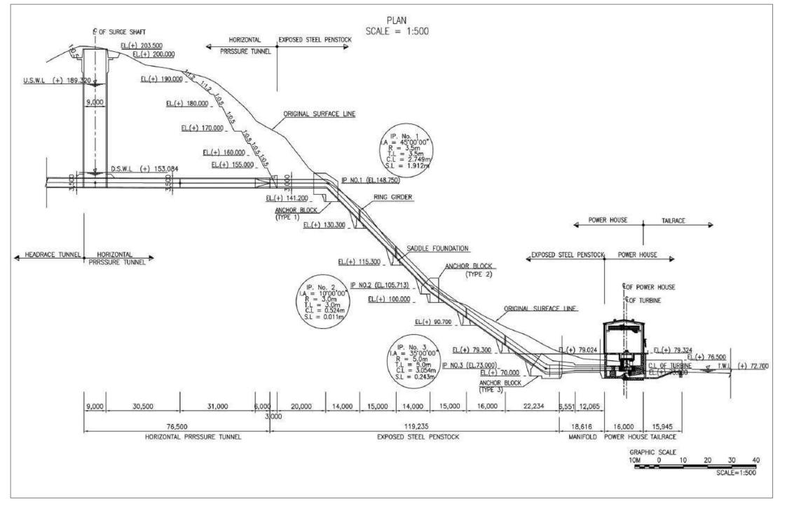
Figure 2-14 Tunnel longitudinal section
