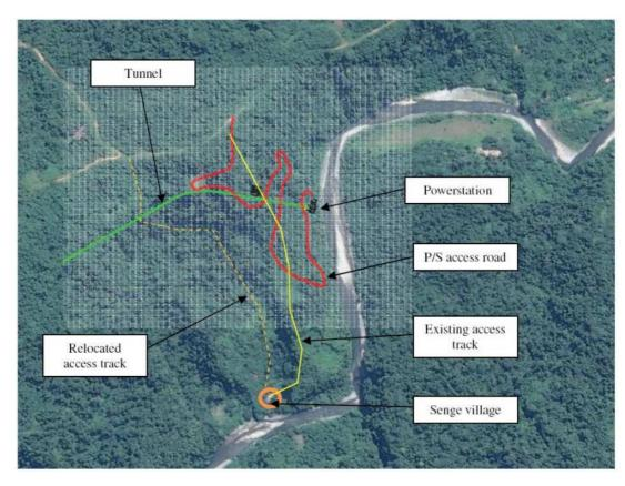
Figure 12-8 Relocation of the footpath to Sengue
