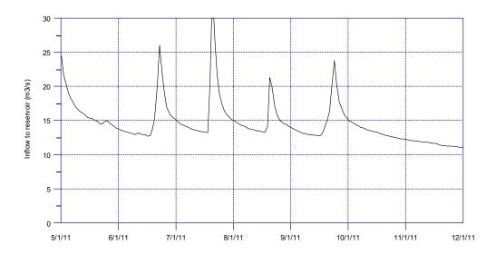
**Figure 11**: Example of inflow sequence that triggers short duration spill events over a number of days.
