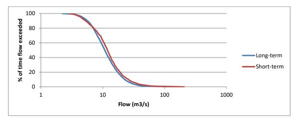
Figure 8: Flow duration curves for long-term synthetic flows in the Tina River at dam site (2010-2014) and short-term recorded flows (16 June 2010 to 3 April 2014).
