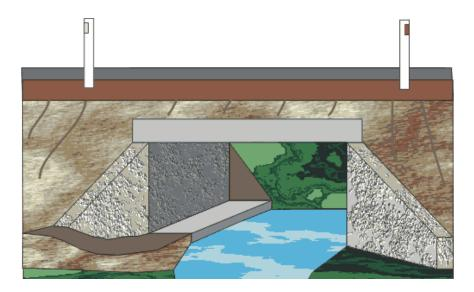
Figure 13-1 Culvert with dry passage for reptiles
