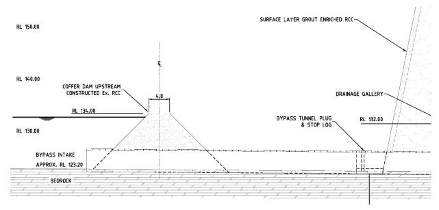
Figure 2-8 Diversion by-pass intake and by-pass plug
