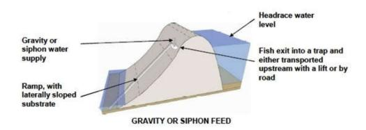
Figure 11-3 shows the trap system with ramp leading to a holding tank and piped water supply installed at Waitaki Dam, New Zealand. The ramp can be lined with bristles, gravel or a drainage product called Miradrain or Cordrain (Patterson & Boubee 2010). The optimum slope is about 15 degrees.
