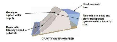
Figure 16: Principle of trap and transfer system
