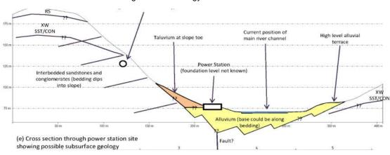
Figure 2-10 Geology at the Powerhouse site
