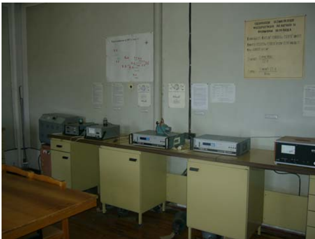
Figure 6.18 – Gas analyzers to detect and determine the content of carbon monoxide and hydrocarbons
