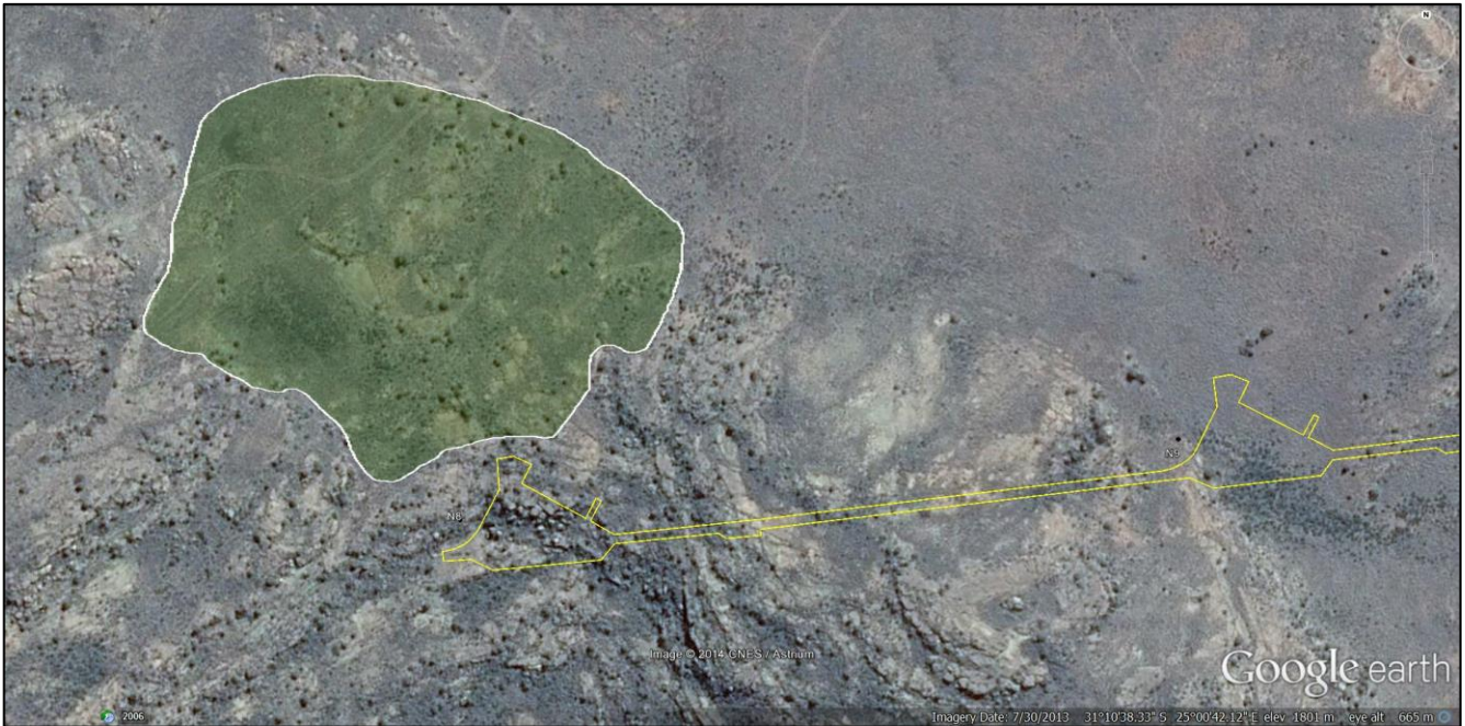
Figure 6. The location of Turbine 8, illustrating the rocky nature of the current location. The green-highlighted area indicates the closest suitable area where the turbine might be moved to.
