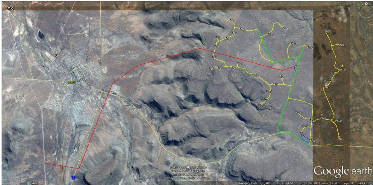
Figure 1. Satellite image illustrating the layout of the Noupoot Wind Energy Facility, with power line in red, existing roads in green, new turbine access roads in yellow and laydown area, substation and control buildings in blue.
