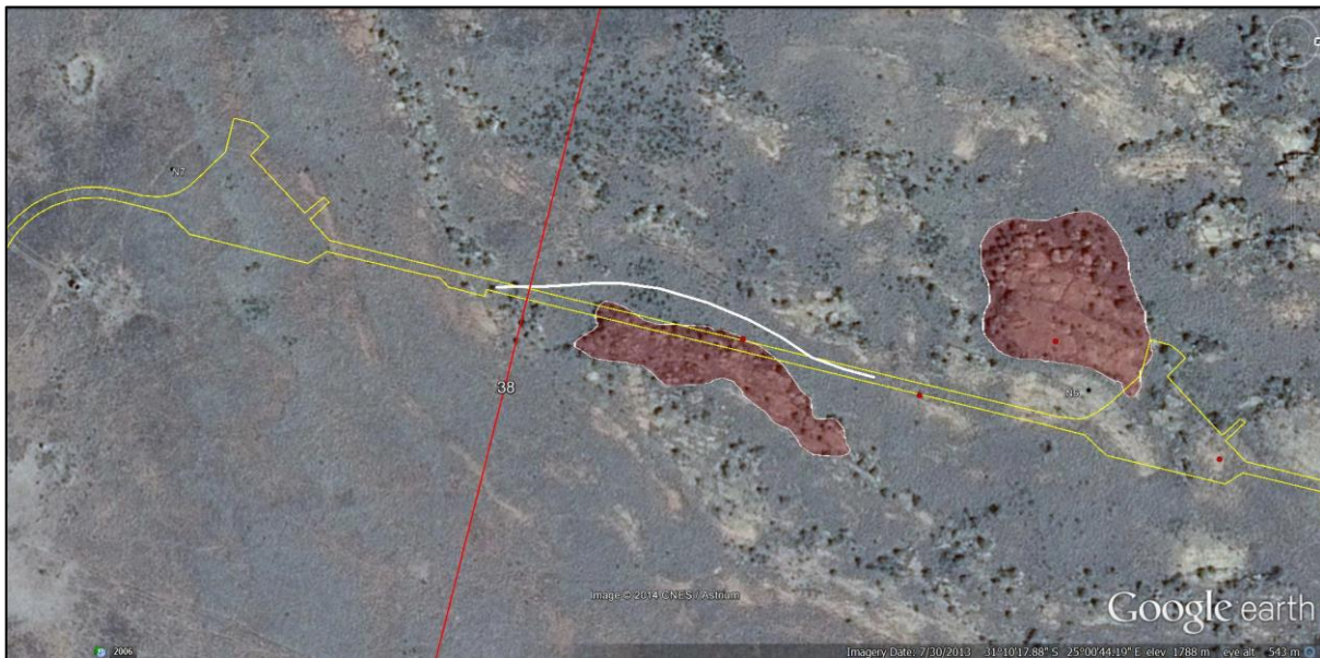
Figure 3. Satellite image showing the sensitive ridge habitat along the access road between Turbines 6 and 7, and the recommended alternative route in white. The image also illustrates the location of the rock platform with freshwater pools near to Turbine 6. This area should be avoided as the pools are not a common feature in the area. Note that the orientation of the map is with north to the right.
