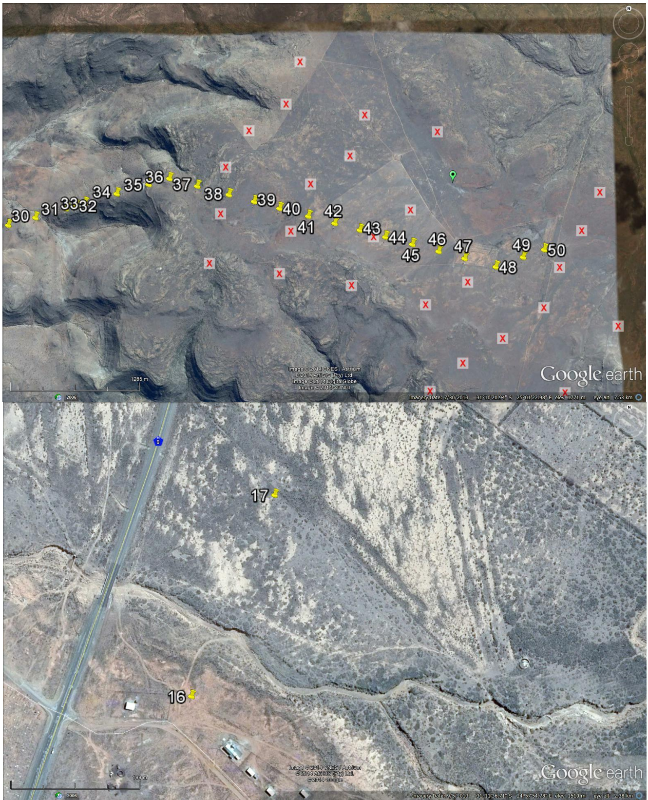
Figure 4: The sections of 132kV line that requires marking with BFD's.
