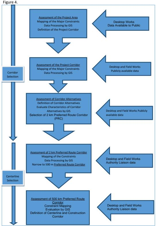
**Figure 4 Route Selection Process Workflow**
