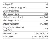
**Standard equipment** (R18ID3-0 1 x impact bit, 1 x 5/8 inch socket adpator
