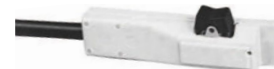
RMLS-14 (14-pin plug) 129337 Momentary- and maintained-contact rocker switch for contactor control. Push forward for maintained contact and backward for momentary contact. Includes 26.5-foot (8 m) cord with plug.
