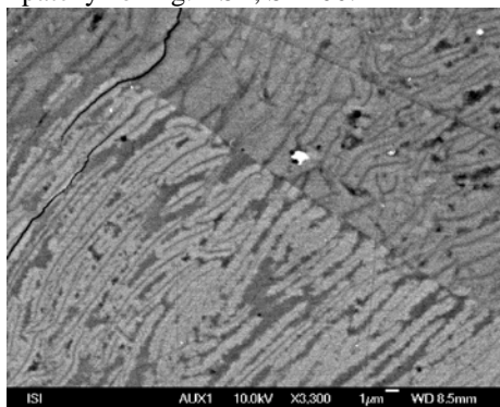
Fig.3. Close-up of the perlitic texture, overprinted by alteration and recrystallization. FEG-SEM, Jeol.
