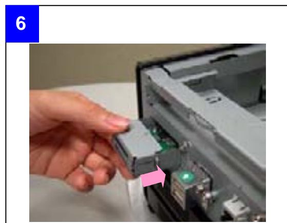
■ Install the assembled Card Reader back to the chassis with attach screw
