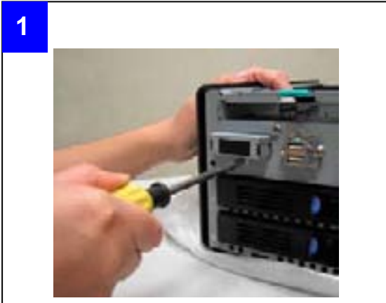
■ Detached the front screw of Card Reader holder
