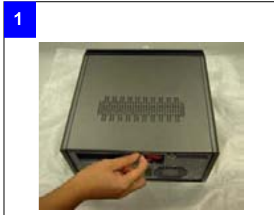
■ Release the side panel thumb screw on the rear
