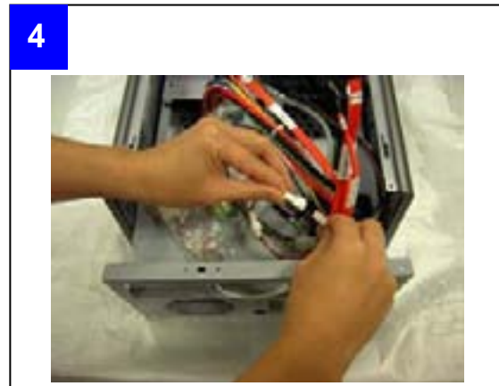
■ Disconnect the extension fan cables
