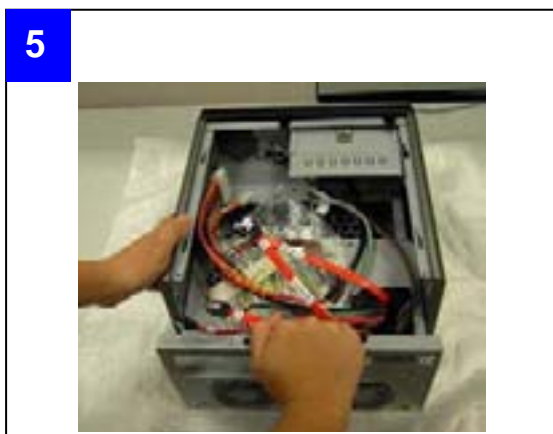
■ Detach the motherboard cage with System Cables (SATA, Power, Fan cables) through the cable routing hole
