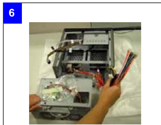
■ Finish detaching the M/B cage and make sure all the connection on backplane and PDB are still tight before assembly back the M/B cage
