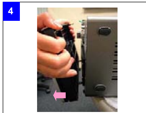
■ gently pull the bezel to make it detach
