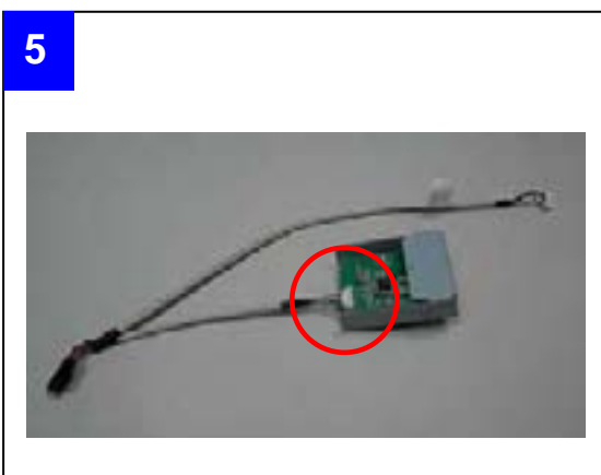
■ Connect the short end of USB split cable to Card Reader with
