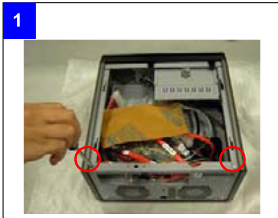
■ Release the secure screws on the M/B cage
