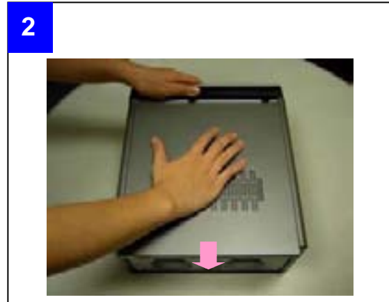
■ Push and slide the side panel toward rear to open the chassis
