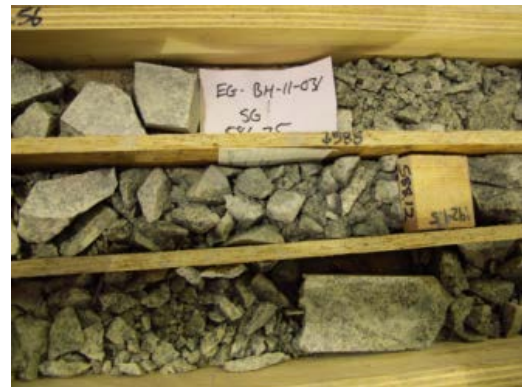
SG sample – hole BH-11-031 @ 586.75 m
