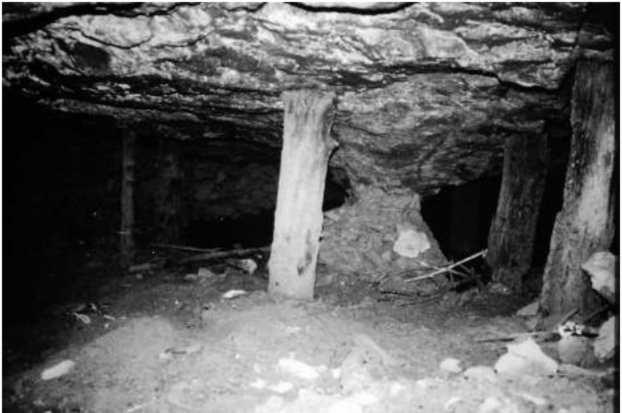
A view inside the mine showing timber props from World War I, a pack wall to the left, and a pillar with chrome ore. (Author's photograph, 30 August 1997.)
