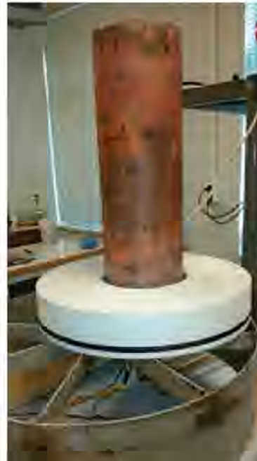
Figure 2.7. From Figure 2-1 in TR 15-09. The test set-up, which to a certain extent is a model of a KBS-3 deposition hole. Mounted on a plastic plate is a copper tube which is heated by circulating water to approximately 80 °C. “Water injection” seen to the left is actually a hole for low pressure water vapour to enter the slot between the Cu-heater and the bentonite rings. The outside of the set-up was covered by a plexiglass tube (not visible here).
