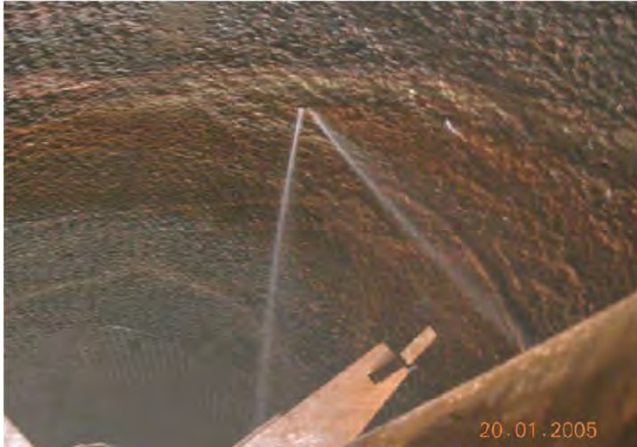
Figure 2.2. From Figure 3 in SKB-report R-05-44. Typical inflow pattern in Äspö hard rock laboratory showing high pressurized groundwater seeping out of a drilled rock surface. This photo is taken from a depth of only 220 m, i.e. the water pressure is around 22 bar, only half of that prevailing in a real repository. The cracks in the deposition holes in Forsmark are believed to be smaller but the pressure of the ground water is still 50 bar.
