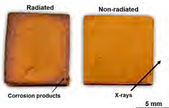
Figure 5.2. Photograph of some of the copper samples to be investigated. The radiated specimen in this case was exposed to oxygen-free water for 64 hours with a simultaneous exposure to 28.6 kGy of gamma radiation. The non-radiated specimen was exposed to oxygen-free water for 64 hours only. The bar shows the scan direction of x-rays through the specimen.
