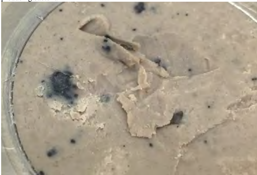
Black colonies of iron sulphide produced by sulphide producing bacteria observed during sampling of test cell with GMZ bentonite.
