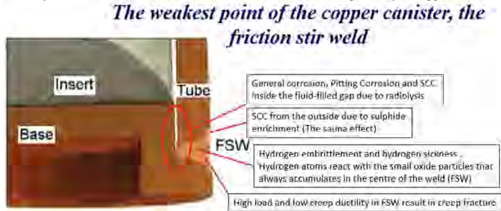
Figure 3.11. Detail from /Szakálos P. et al. 2017/. The weakest point of the canister is the Friction Stir Weld (FSW) and the fastest degradation mechanism is “hydrogen sickness” in the welds.
