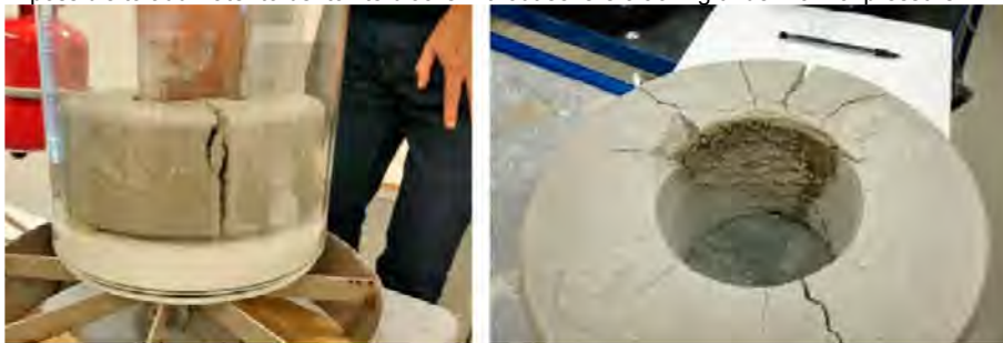
Figure 2.6. From Figure 2-8 in SKB TR-15-09. Left: Test 3 at termination. Right: Bottom side of the bentonite ring showing a condensation “nucleus” and cracks. Severe cracking of the bentonite rings occurred already within 7 days, which was the experiment duration time.
