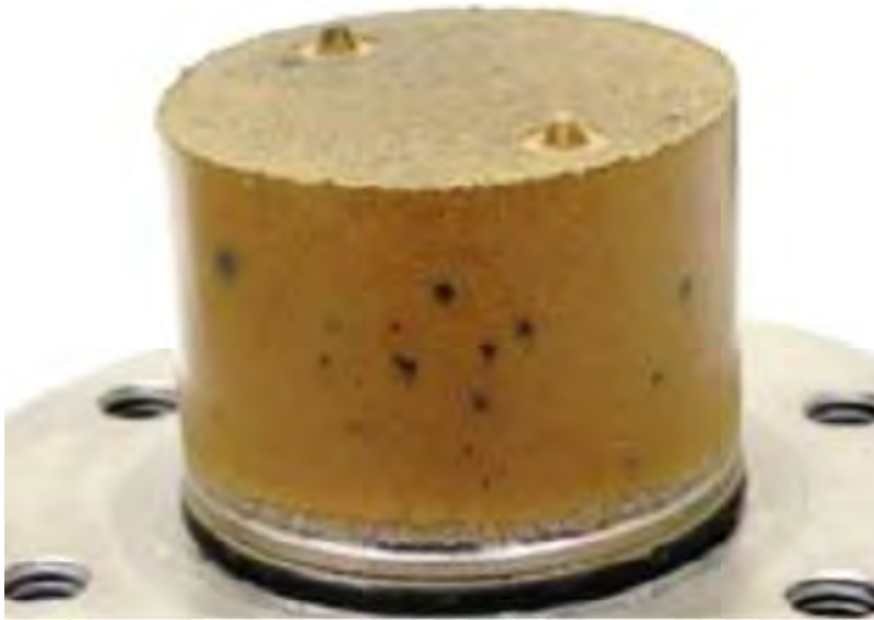
Black colonies of iron sulphide produced by sulphide producing bacteria in Asha bentonite at 1750 kg/m 3 wet density and with addition of lactate and sulphide producing bacteria
