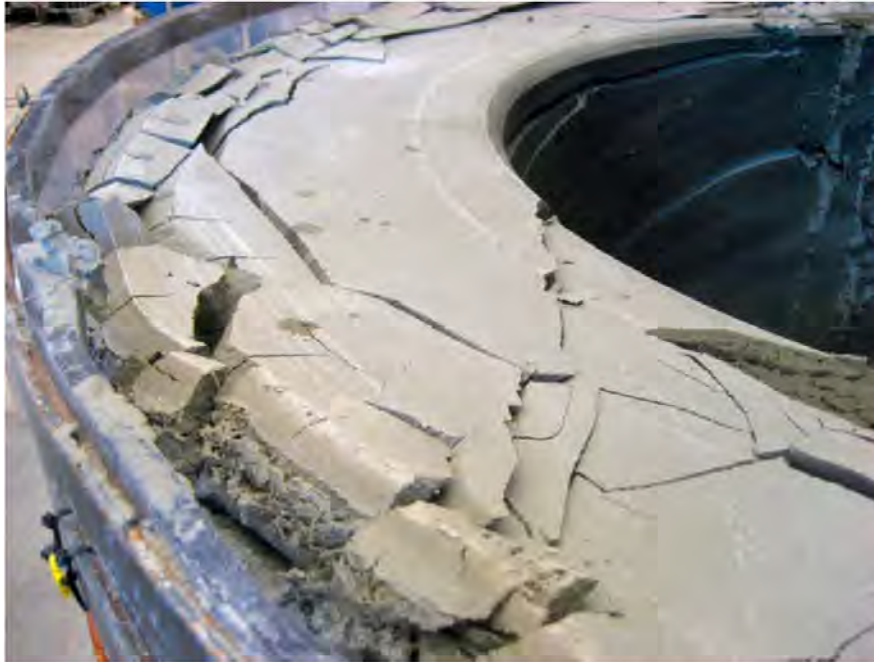
Figure 2.5. From SKB-report TR-17-15, Fig 2.9. SKB has shown in several reports that it is impossible to add water to bentonite blocks without severe cracking under normal pressure.
