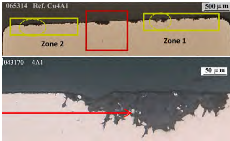
Figure 4.6. Metallographic cross-sections showing the exposed copper sample with pitting corrosion, up to 100μm in depth. From Appendix B in the FEBEX-report /Wersin P. and Kober F 2017/.
