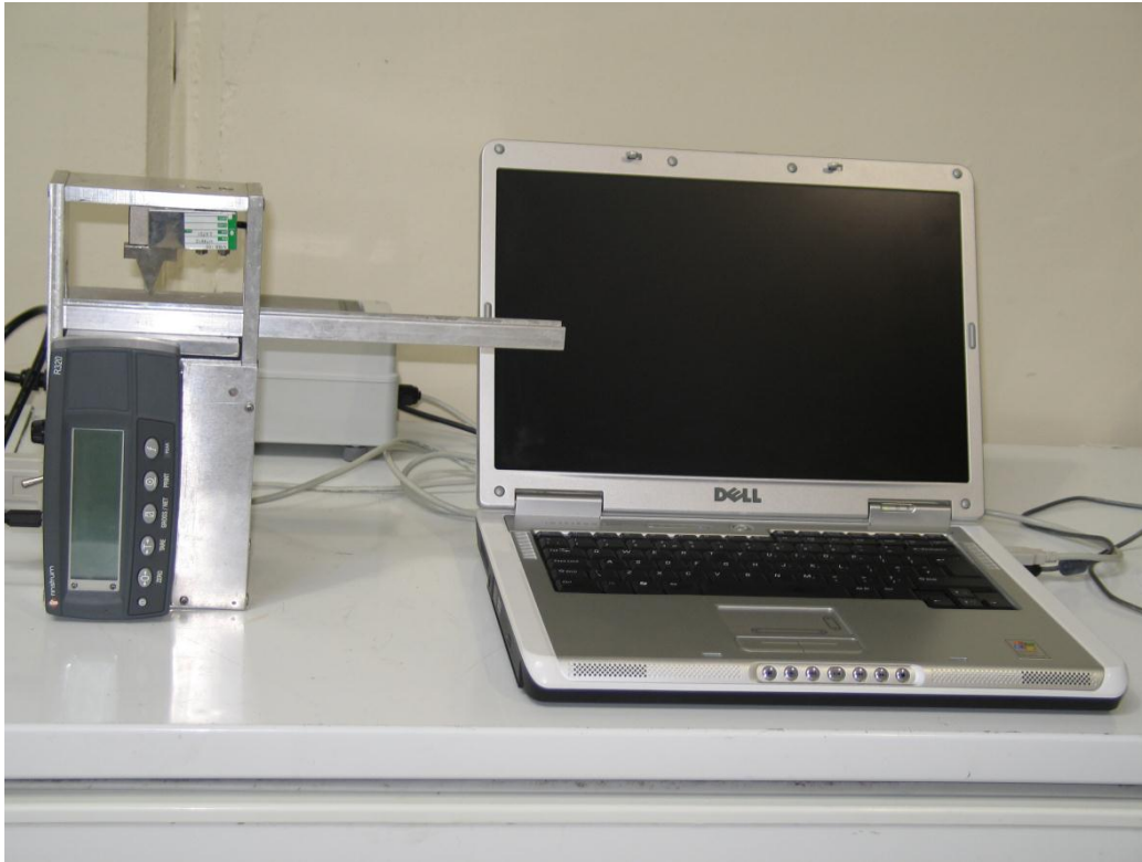
Photograph A1 - A photograph of the new G2 prototype Tenderometer connected to a laptop PC.
