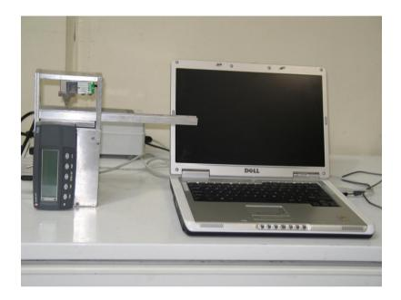
Figure 5. The G2 Tenderometer connected to a laptop PC for automatic data capture
