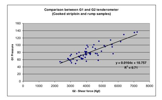
Figure 7. Comparison in shear force between G1 and G2 tenderometers
