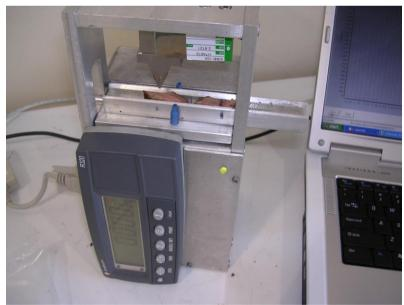
Figure 6. View of G2 Tenderometer from above. This photograph clearly shows the raised platform with the presentation tray moving the samples up to the shearing tooth.
