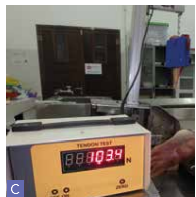
Figure 4. Achilles tendon secured onto a tensile testing machine (A, B). The monitor showed the ultimate strength (C).
